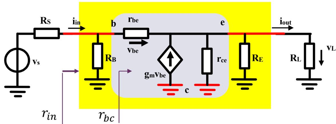
$$G_p = \frac{P_L}{P_{in}} = \frac{v_L i_{out}}{v_{in} i_{in}} = \frac{v_L v_S i_{out}}{v_S v_{in} i_{in}} = 0.972 \times \frac{r_{in} + R_S}{r_{in}} \times 9.417$$
