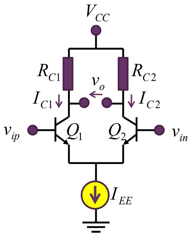
$$v_o = (V_{CC} - I_{C2}R_{C2}) - (V_{CC} - I_{C1}R_{C1})$$
