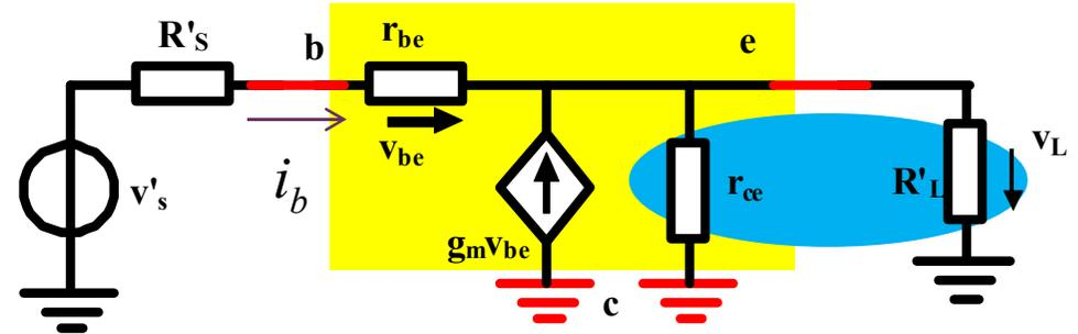
$$v'_S = i_b (R'_S + r_{be}) + (i_b + g_m r_{be} i_b) R''_L$$
