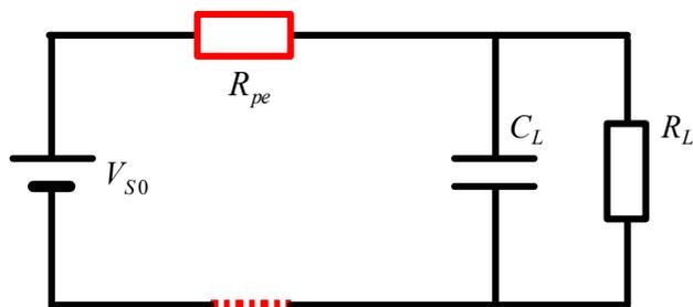
$$\Delta V \stackrel{C_L \gg C_p}{\approx} \frac{R_{pe}}{R_L + R_{pe}} \frac{C_p}{C_L} V_{S0}$$
