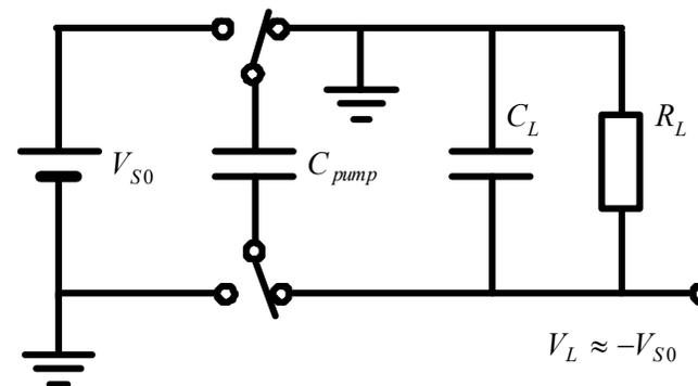
$$v_o(t) = V_1 e^{-\frac{t}{R_L(C_L + C_p)}} \approx V_1 \left( 1 - \frac{t}{R_L(C_L + C_p)} \right)$$
