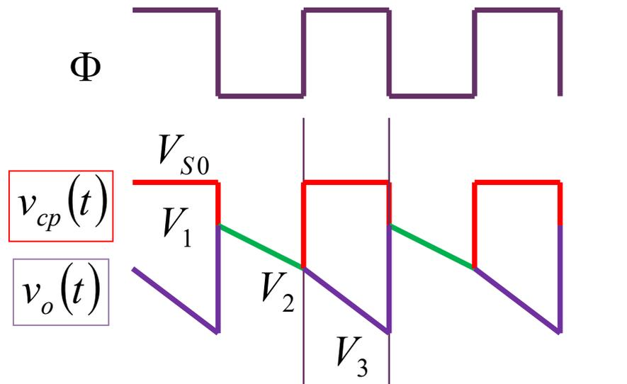
$$V_1 \approx \frac{C_p}{C_p + C_L} \frac{V_{S0}}{\frac{0.5T}{R_L \left( (C_L + C_p) \text{串} C_L \right)}}$$
