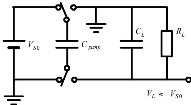
$$C_L \gg C_p \quad R_{pe} = \frac{T}{C_p}$$
