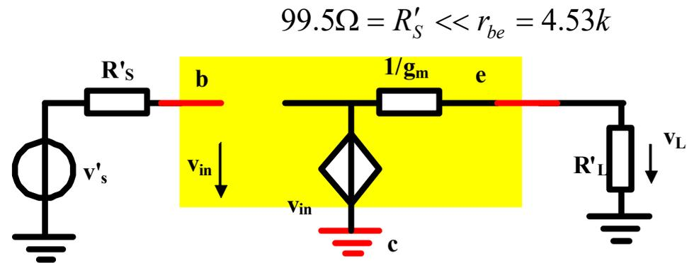
$$v_L = \frac{R'_L}{R'_L + \frac{1}{g_m}} v'_S = \frac{g_m}{1 + g_m R'_L} R'_L v'_S = g_{mf} R'_L v'_S$$
