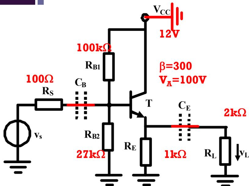
$$v'_S = \frac{R_B}{R_S + R_B} v_S = \frac{21.3k}{0.1k + 21.3k} v_S = 0.995 v_S$$
