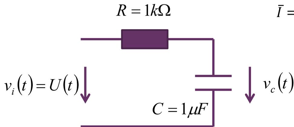
$$\bar{I} = \frac{\Delta Q}{T} = \frac{CV_1 - CV_2}{T} = C \frac{\Delta V}{T} = \frac{\Delta V}{T/C} = \frac{\Delta V}{R_{eff}}$$
