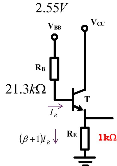
$$I_B R_B + V_{BE} + (\beta + 1) I_B R_E = V_{BB}$$
