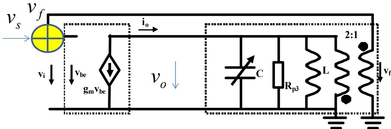
$$A_{vF} = \frac{\dot{V}_o}{\dot{V}_s} = \frac{\dot{V}_o}{\dot{V}_i - \dot{V}_f} = \frac{1}{\frac{\dot{V}_i}{\dot{V}_o} - \frac{\dot{V}_f}{\dot{V}_o}} = \frac{1}{-\frac{1}{\overline{g_m Z_L}} + \frac{1}{n}} = \frac{-\overline{g_m Z_L}}{1 - \overline{g_m Z_L} \frac{1}{n}}$$
