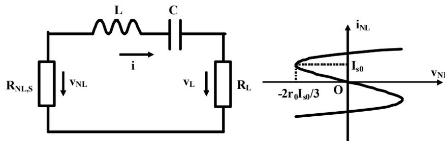
$$\bar{r}_n = r_0 \left( 1 - \left( \frac{I_{m\infty}}{2I_{s0}} \right)^2 \right) = R_L$$
