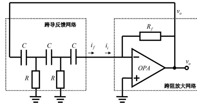
$$T_0 = A_0 F = -R_f \cdot \frac{sC \cdot (sRC)^2}{3s^2 R^2 C^2 + 4sRC + 1} \Big|_{s=j\omega} = R_f \cdot \frac{j\omega C \cdot (\omega RC)^2}{(1 - 3\omega^2 R^2 C^2) + 4j\omega RC} = |T_0(\omega)| e^{j\varphi_T(\omega)}$$
