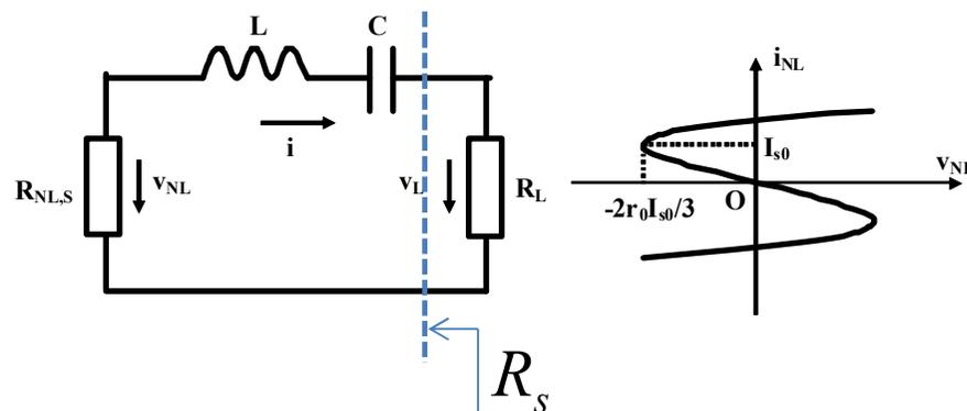
$$v_{NL}(t) = \left( r_0 - r_0 \frac{I_m^2}{4I_{s0}^2} \right) I_m \cos \omega_0 t - \frac{r_0}{12I_{s0}^2} I_m^3 \cos 3\omega_0 t$$
