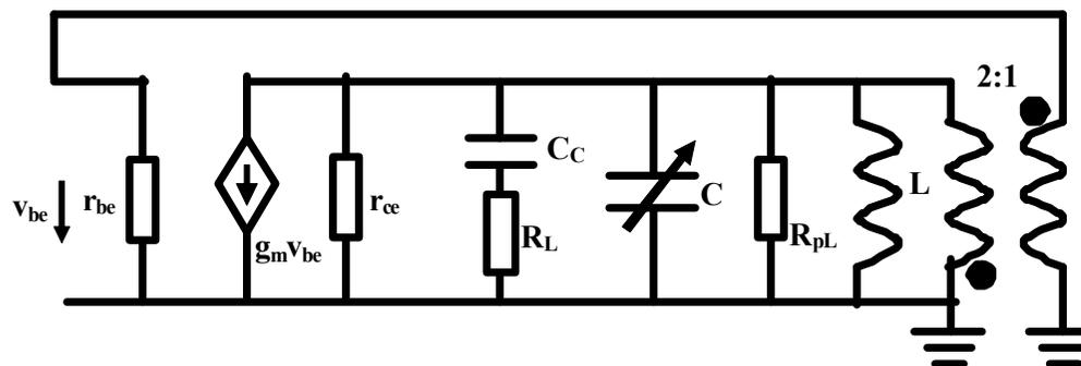
$$C \approx \frac{1}{(2\pi f_0)^2 \times L} = \frac{1}{(2 \times 3.14 \times 2 \times 10^6)^2 \times 30 \times 10^{-6}} = 211 pF$$
