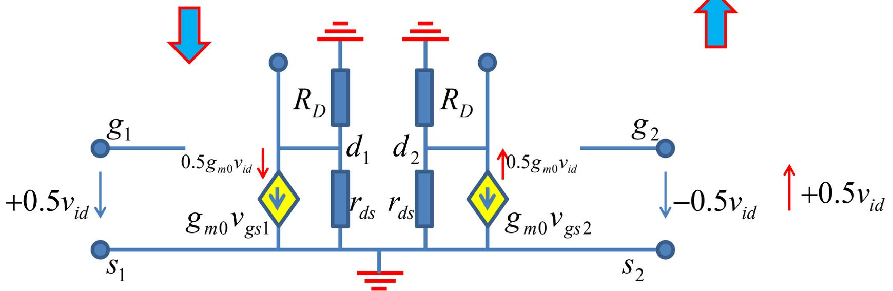
$$g_{m0} = \frac{2I_{D0}}{V_{od0}} = \frac{I_{SS}}{V_{od0}}$$
