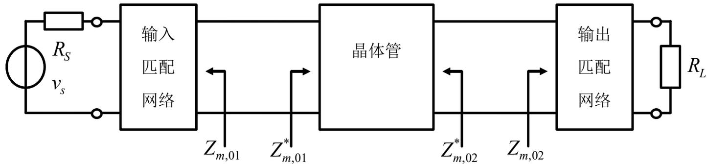
$$k = \frac{2\text{Re}Y_{11}\text{Re}Y_{22} - \text{Re}(Y_{12}Y_{21})}{|Y_{12}Y_{21}|} < 1$$
