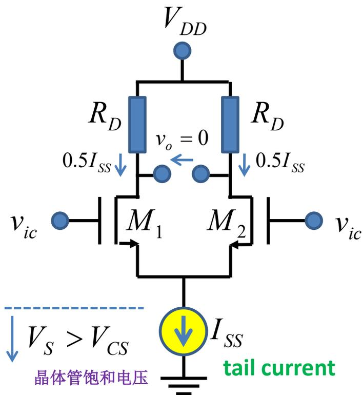
$$v_{ip} = v_{in} = v_{ic}$$
