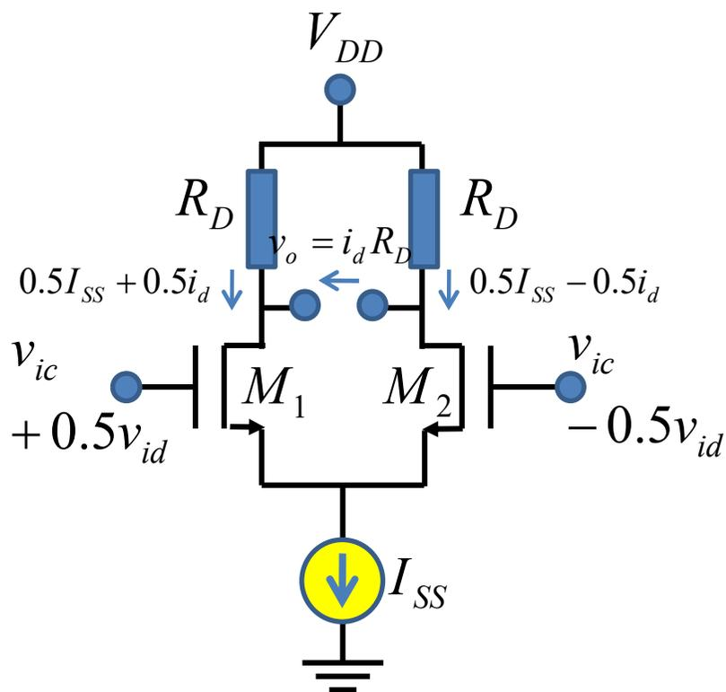
$$V_{GS1} - V_{GS2} = v_{id}$$
