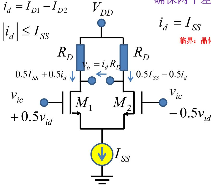
$$i_d = I_{SS} \quad I_{D1} = I_{SS} = \beta_n V_{od1}^2 \quad I_{D2} = 0 = \beta_n V_{od2}^2$$
