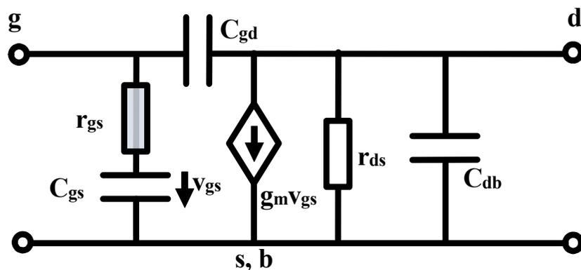
$$f_{\max} = \frac{g_m}{4\pi C_{gs}} \sqrt{\frac{r_{ds}}{r_{gs}}}$$
