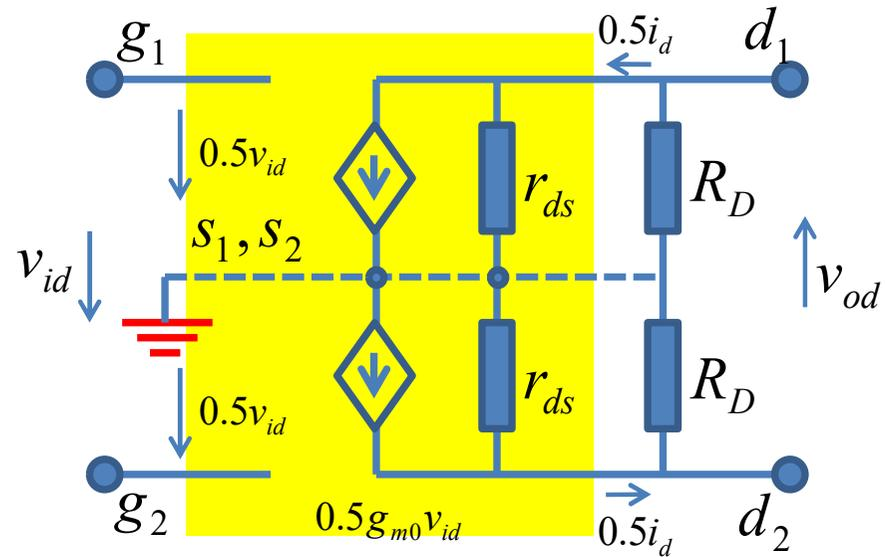
$$v_{od} = 0.5g_{m0}v_{id} \cdot (2r_{ds} \parallel 2R_D) = g_{m0}(r_{ds} \parallel R_D)v_{id}$$
