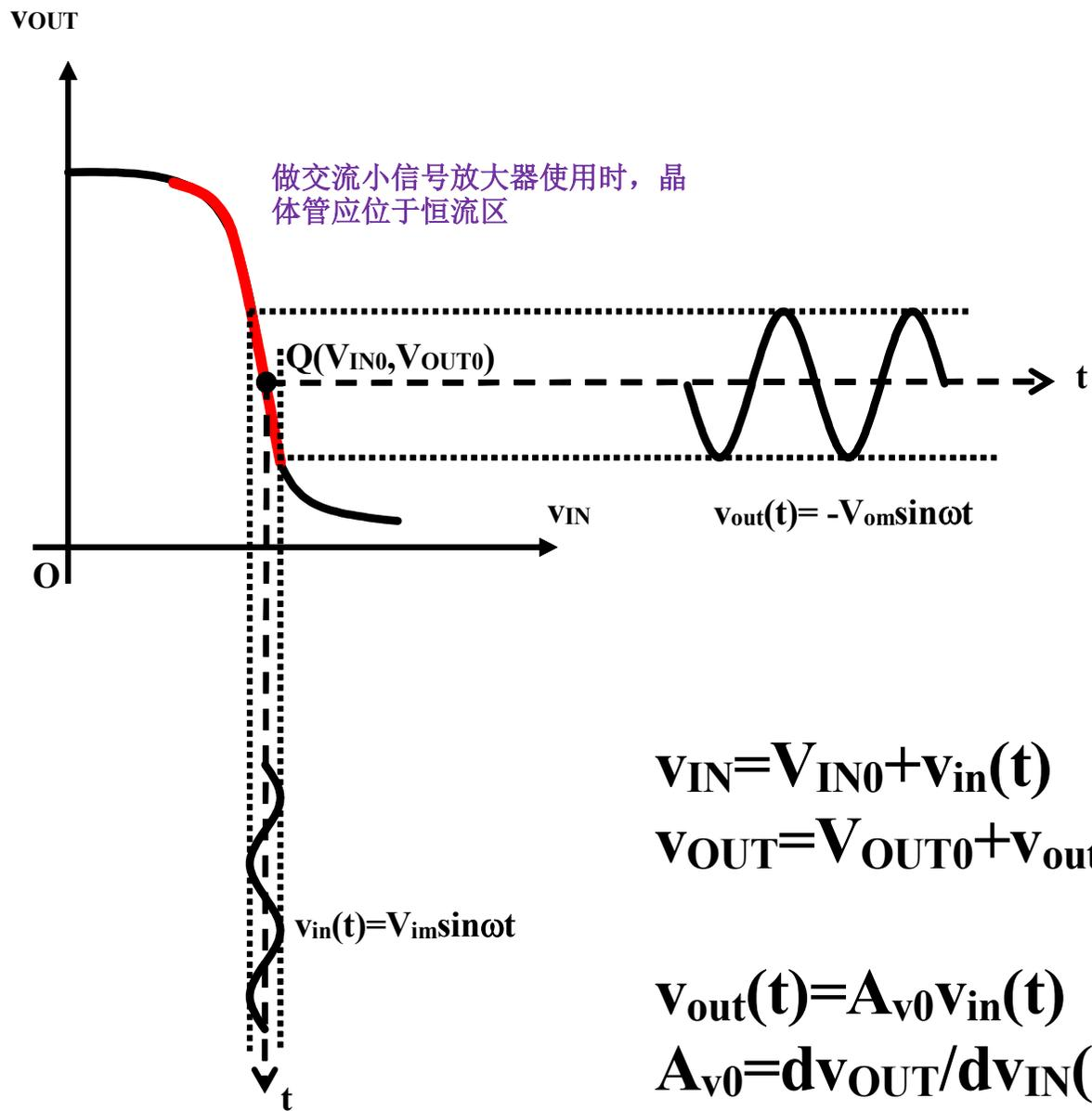
$$V_{IN} = V_{IN0} + v_{in}(t)$$
