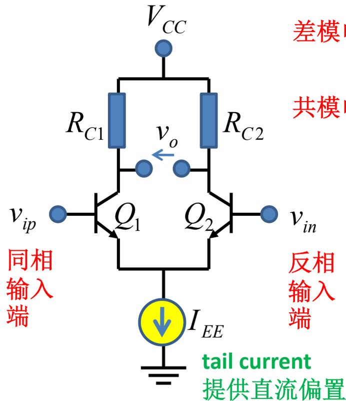
差模电压  $v_{id} = v_{ip} - v_{in}$
