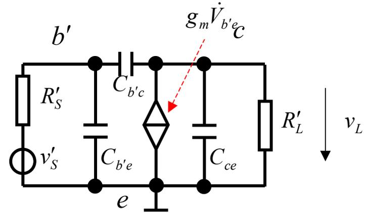
$$A(s) = \frac{v_L}{v'_S} = -g_m R'_L \frac{1 - \frac{s}{\omega_z}}{1 + s(C_{b'e}R'_S + C_{b'c}(R'_S + R'_L + g_m R'_S R'_L) + C_{ce}R'_L) + s^2 R'_S R'_L (C_{b'c}C_{b'e} + C_{b'e}C_{ce} + C_{ce}C_{b'c})}$$
