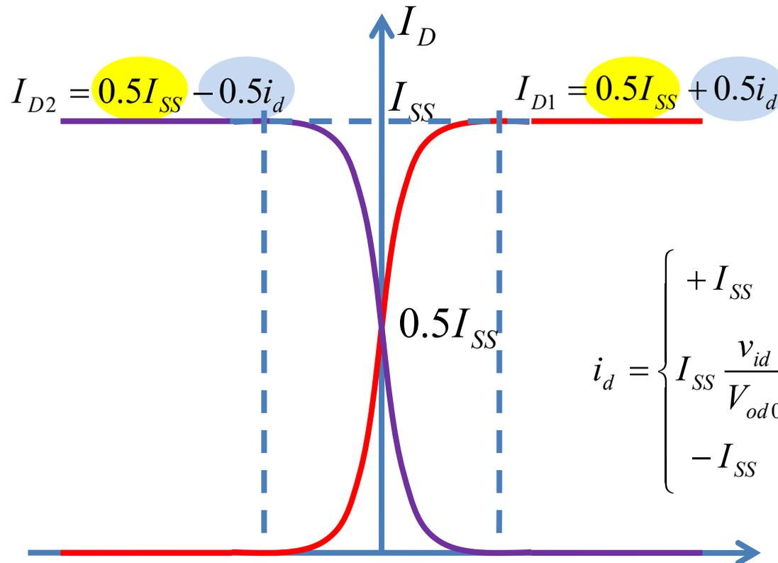
$$i_d = \begin{cases} +I_{SS} & v_{id} \geq +\sqrt{2}V_{od0} \\ I_{SS} \frac{v_{id}}{V_{od0}} \sqrt{1 - \frac{1}{4} \left( \frac{v_{id}}{V_{od0}} \right)^2} & |v_{id}| \leq \sqrt{2}V_{od0} \\ -I_{SS} & v_{id} \leq -\sqrt{2}V_{od0} \end{cases}$$
