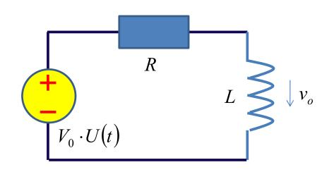
$$v_{L}(0^{+}) = V_{0} \qquad v_{L\infty}(t) = 0$$
