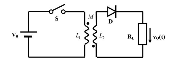
$$i_{L}(t) = \frac{M}{L_{2}} \frac{V_{0}}{L_{1}} t_{0} e^{-\frac{t-t_{0}}{\tau_{2}}} U(t-t_{0}) = \frac{M}{L_{2}} \cdot \frac{V_{0}t_{0}}{L_{1}} \cdot e^{-\frac{t-t_{0}}{\tau_{2}}} U(t-t_{0})$$
