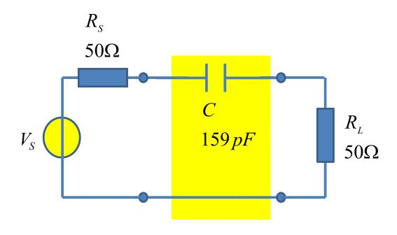
$$C = \frac{\tau}{R_L + R_S} = \frac{1}{2\pi \cdot f_{3dB} \cdot (R_L + R_S)} = \frac{1}{2 \times 3.14 \times 10M \times (50 + 50)} = 159 \, pF$$
