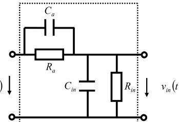
$$H(j\omega) = \frac{\dot{V}_{in}}{\dot{V}_{s}} = \frac{R_{in}||C_{in}}{R_{a}||C_{a} + R_{in}||C_{in}}$$
