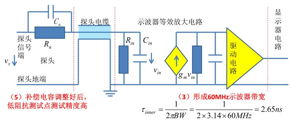
$$au_{in} = (R_{in} \parallel R_a)C_{in} = (1M\Omega \parallel 9M\Omega) \times 10pF = 9\mu s$$
