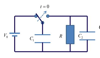
$$V_{C1}(0^{-}) = V_{0} \qquad V_{C2}(0^{-}) = 0$$
