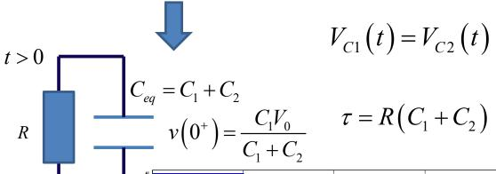
$$V_{C1}(t) = V_{C2}(t) = \frac{C_1 V_0}{C_1 + C_2} e^{-\frac{t}{\tau}}, t > 0$$
