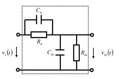
$$v_{in}\left(0^{+}\right) = \frac{C_a}{C_{in} + C_a} V_{S0}$$
