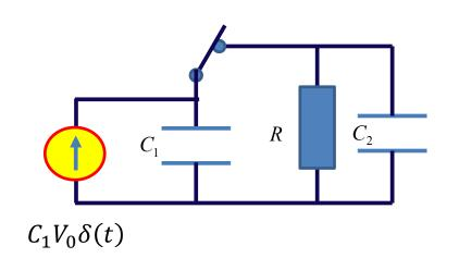
$$V_{C1}(0^{+}) = V_{C2}(0^{+}) = \frac{1}{C_{1} + C_{2}} \int_{0^{-}}^{0^{+}} C_{1}V_{0}\delta(t)dt$$
