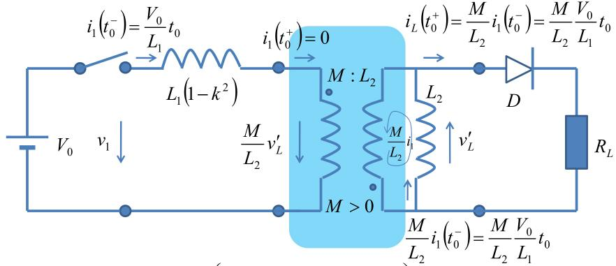
$$v_1(t) = -(1 - k^2)V_0t_0\delta(t - t_0) + \frac{M}{L_2} \cdot \left(-\frac{M}{L_2}\frac{V_0}{L_1}t_0R_Le^{-\frac{t - t_0}{\tau_2}}U(t - t_0)\right)$$
