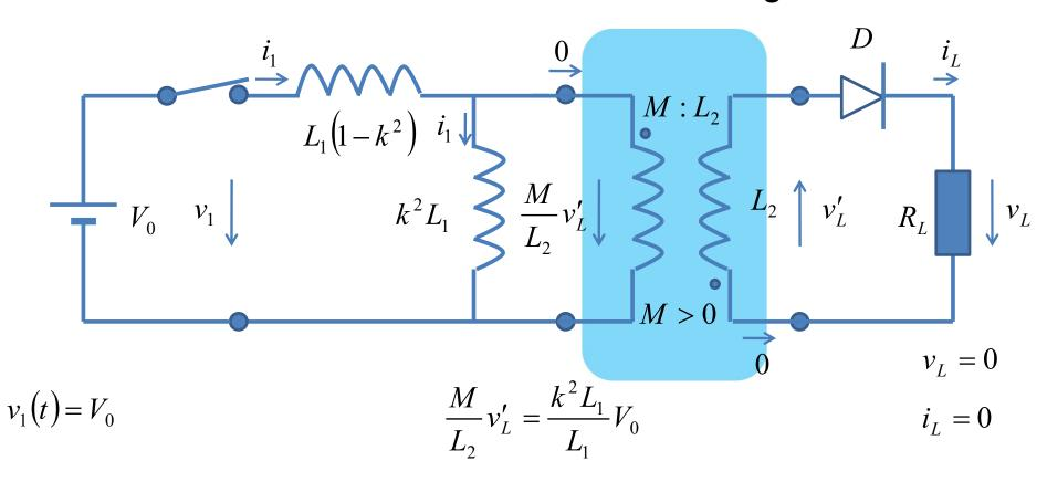
$$i_1(t) = I_{01} + \frac{1}{L_1} \int_0^t v_1(t) dt = \frac{V_0}{L_1} t$$
