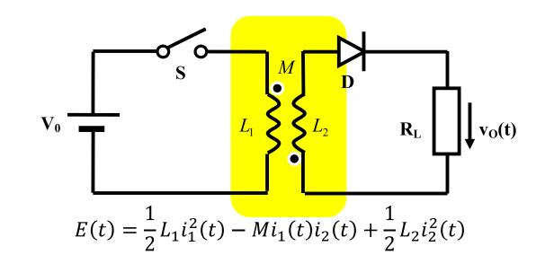
$$E(t) = \frac{1}{2}(1 - k^2)L_1 \cdot i_1^2(t) + \frac{1}{2}L_2 \cdot \left(i_2(t) - \frac{M}{L_2}i_1(t)\right)^2$$
