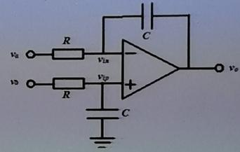
$$v_o(t) = \begin{cases} 0 & t \leq 0 \\ (V_{0b} - V_{0a}) \frac{t}{\tau} & 0 \leq t \leq T \\ \text{sgn}(V_{0b} - V_{0a}) \cdot V_{sat} & t \geq T \end{cases}$$
