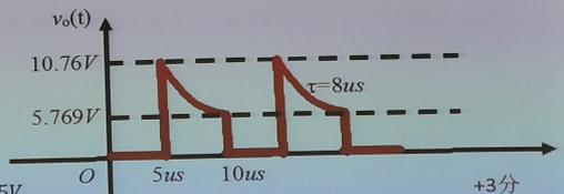
$$V_0 \cdot \frac{RT}{2\sqrt{L_1L_2}} \cdot \frac{e^{-\frac{0.5T}{\tau}}}{1 - e^{-\frac{0.5T}{\tau}}} = 5 \times \frac{0.5353}{1 - 0.5353} = 5.769V \quad \text{本题共15分}$$
