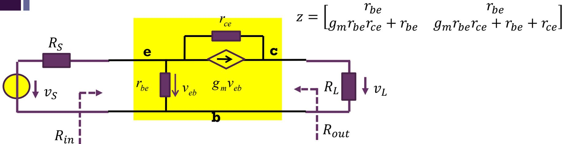
$$z = \begin{bmatrix} r_{be} & r_{be} \\ g_m r_{be} r_{ce} + r_{be} & g_m r_{be} r_{ce} + r_{be} + r_{ce} \end{bmatrix}$$
