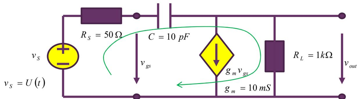
$$\left(R_S + \frac{1}{sC} + R_L\right) \dot{I}_l = \dot{V}_s + g_m \dot{V}_{gs} R_L = \dot{V}_s + g_m (\dot{V}_s - R_S \dot{I}_l) R_L$$
