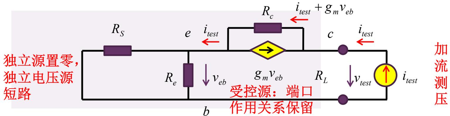
$$v_{test} = (i_{test} + g_m v_{eb}) R_c + v_{eb} = i_{test} R_c + (g_m R_c + 1) v_{eb}$$
