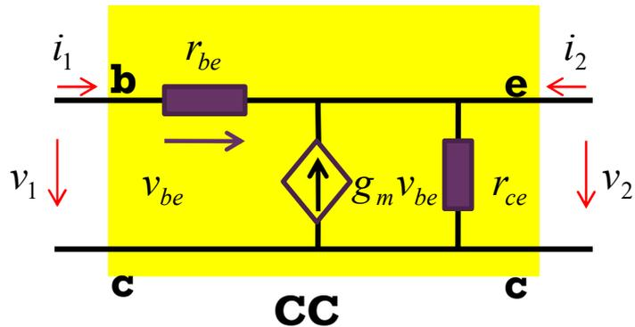
$$\begin{aligned} v_2 &= r_{ce}(i_2 + i_1 + g_m v_{be}) = r_{ce}(i_2 + i_1 + g_m r_{be} i_1) \\ &= (1 + g_m r_{be}) r_{ce} i_1 + r_{ce} i_2 \end{aligned}$$
