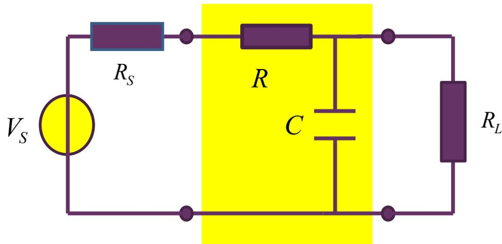
$$H(j\omega) = 2 \sqrt{\frac{R_S \dot{V}_L}{R_L \dot{V}_S}} = H_0 \frac{\omega_0}{s + \omega_0}$$
