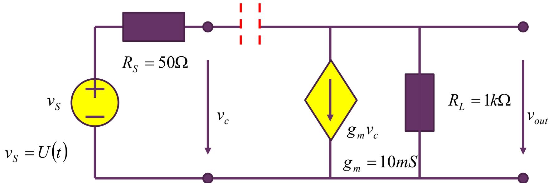
$$v_{out}(t) = -g_m R_L v_S(t) = -10U(t)$$
