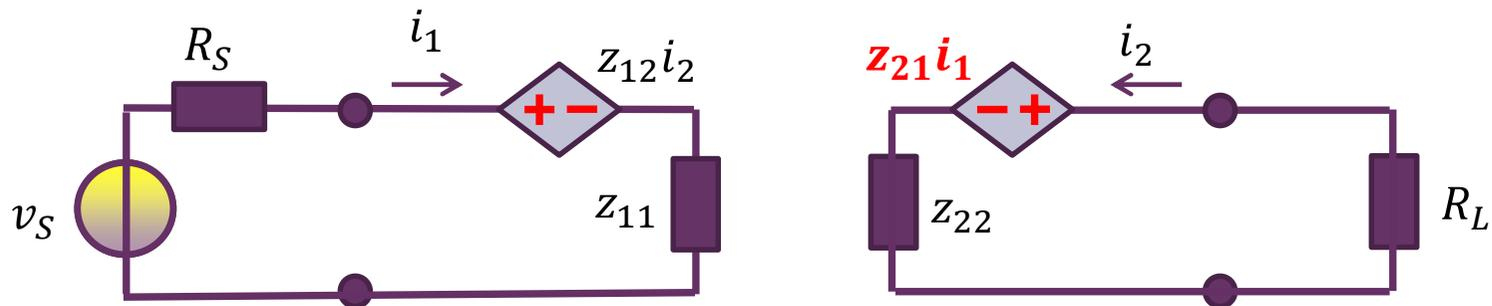
$$H = \frac{-z_{21} R_L}{z_{21} z_{12} - (R_L + z_{22})(R_S + z_{11})}$$
