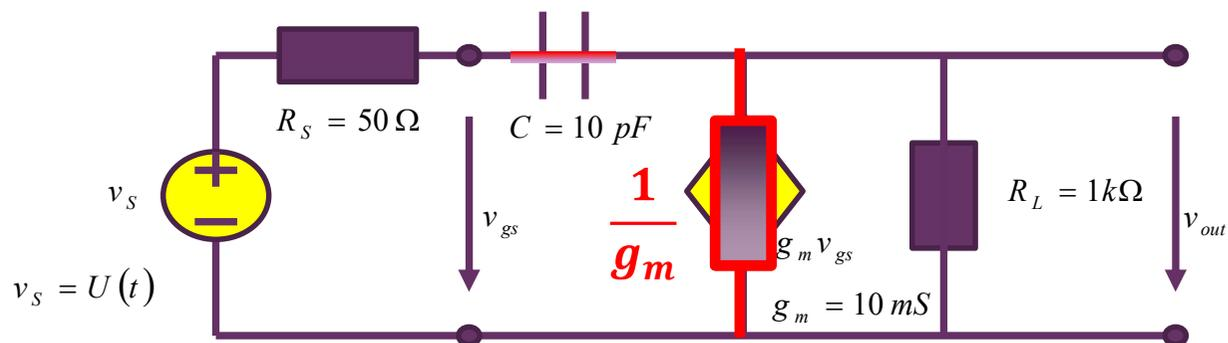
$$v_o(0^+) = \frac{R_L \parallel \frac{1}{g_m}}{R_S + R_L \parallel \frac{1}{g_m}} v_s(0^+) = \frac{\frac{R_L}{1 + g_m R_L}}{R_S + \frac{R_L}{1 + g_m R_L}} v_s(0^+)$$
