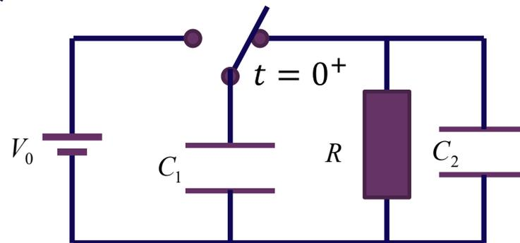
$$v_{C_1}(t) = v_{C_2}(t) = \frac{C_1}{C_1 + C_2} V_0 e^{-\frac{t}{\tau}} \quad (t > 0)$$
