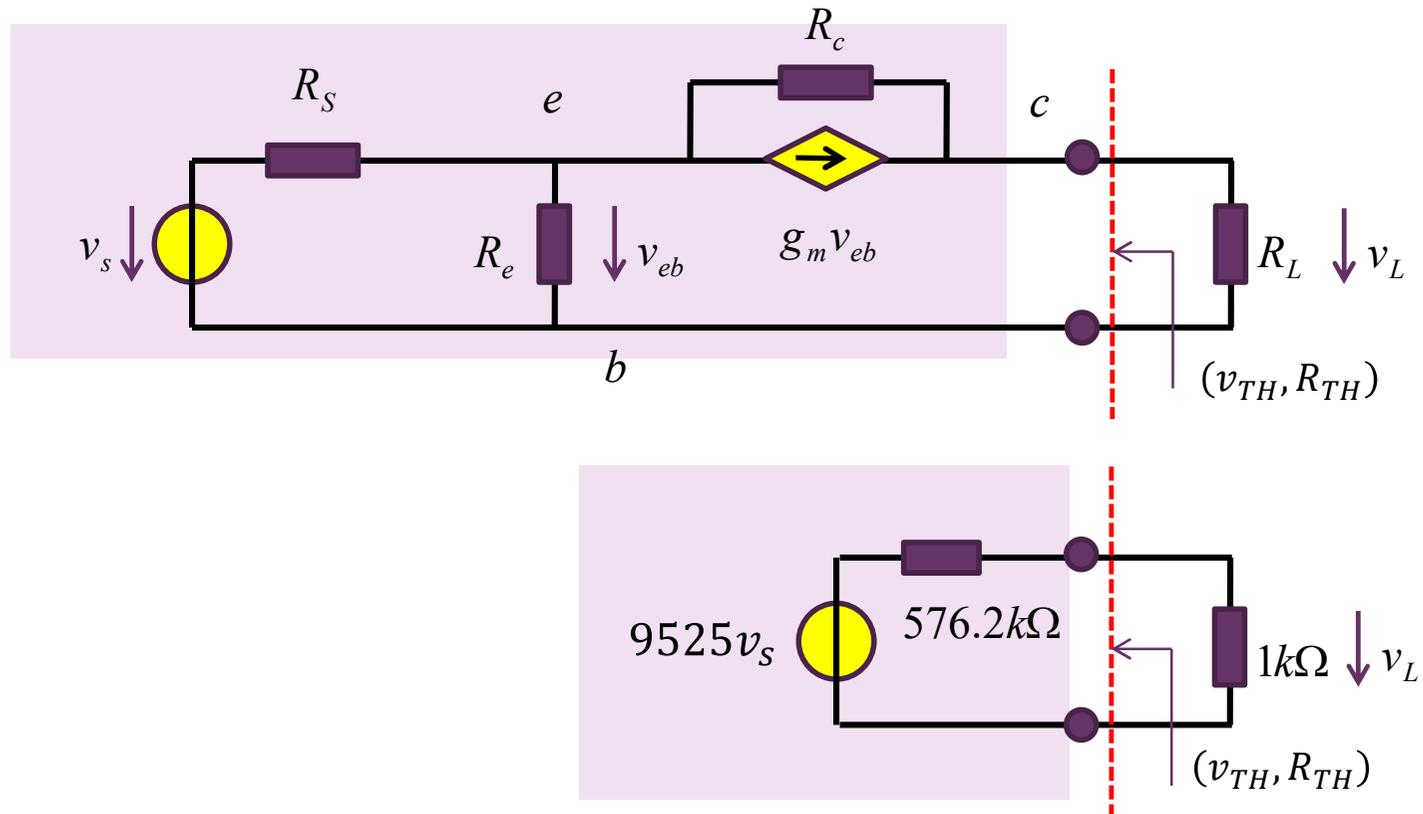
$$v_L = \frac{R_L}{R_{TH} + R_L} v_{TH} = \frac{1k}{576.2k + 1k} \times 9525v_s = 16.50v_s$$
