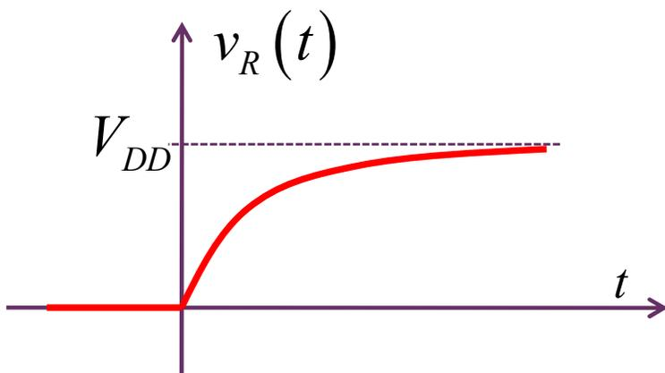
$$i_L(t) = \frac{V_{DD}}{R} \left( 1 - e^{-\frac{t}{GL}} \right) U(t)$$
