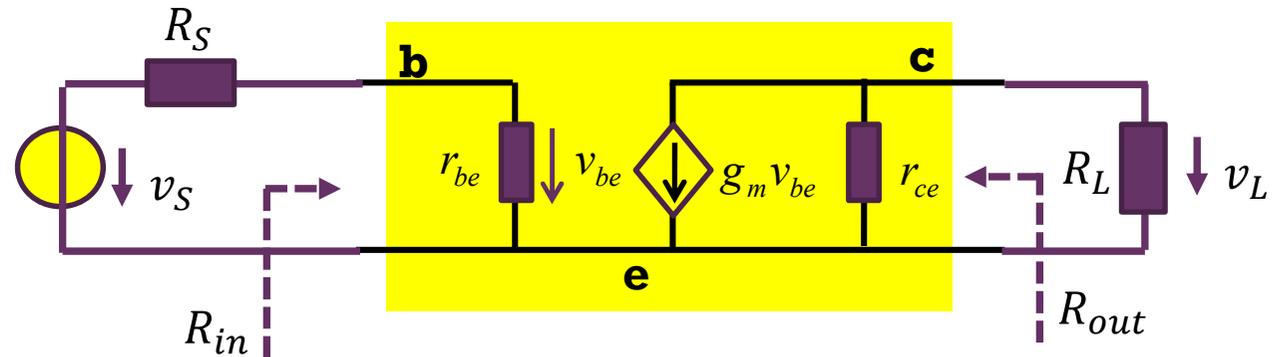
$$R_{in} = r_{be} = 10k\Omega$$
