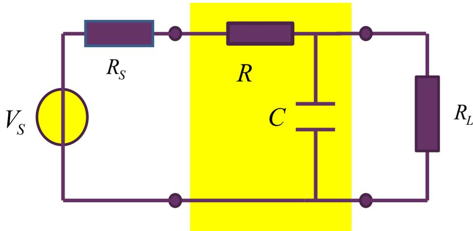
$$H(j\omega) = 2 \sqrt{\frac{R_S}{R_L}} \frac{\dot{V}_L}{\dot{V}_S}$$
