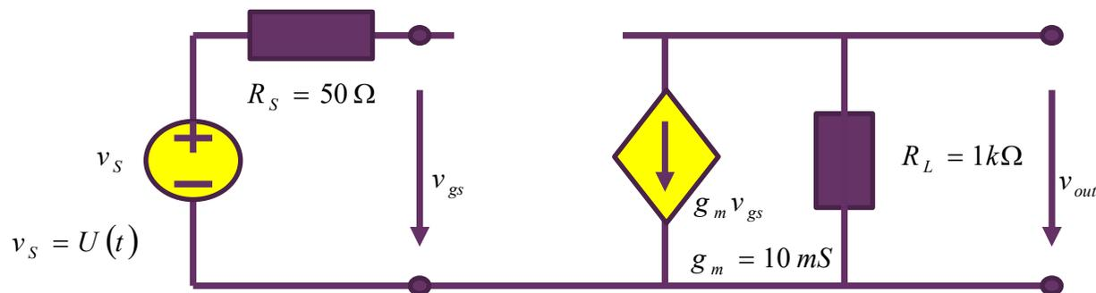
$$v_{o\infty}(t) = -g_m R_L v_{s\infty}(t) = -10 \text{ m} \times 1 \text{ k} \times 1 = -10 \text{ V}$$
