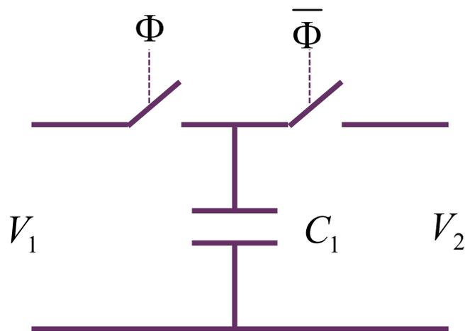
$$\Phi \quad Q_{\Phi} = C_1 V_1$$
