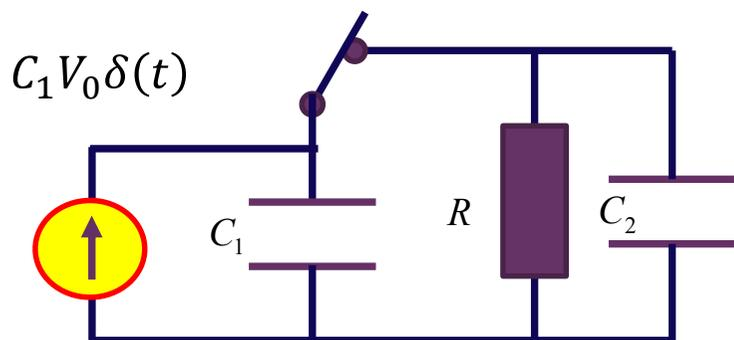
$$v_o(0^+) = \frac{1}{C_1 + C_2} \int_{0^-}^{0^+} C_1 V_0 \delta(t) dt \\ = \frac{C_1 V_0}{C_1 + C_2} \int_{0^-}^{0^+} \delta(t) dt = \frac{C_1 V_0}{C_1 + C_2}$$
