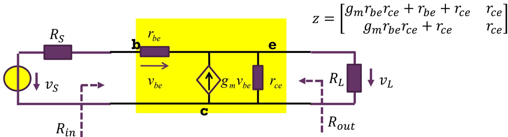
$$R_{in} = z_{in} = z_{11} - \frac{z_{12}z_{21}}{z_{22} + R_L} = g_m r_{be} r_{ce} + r_{be} + r_{ce} - \frac{r_{ce}(g_m r_{be} + 1)r_{ce}}{r_{ce} + R_L}$$
