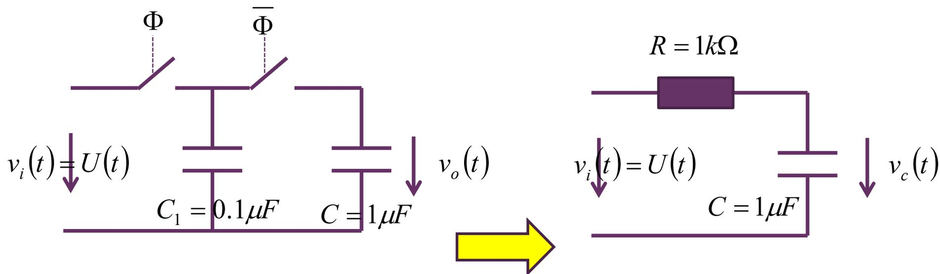
$$v_{C2}(n) = \left( 1 - \left( \frac{C_2}{C_1 + C_2} \right)^n \right) \cdot U(n)$$
