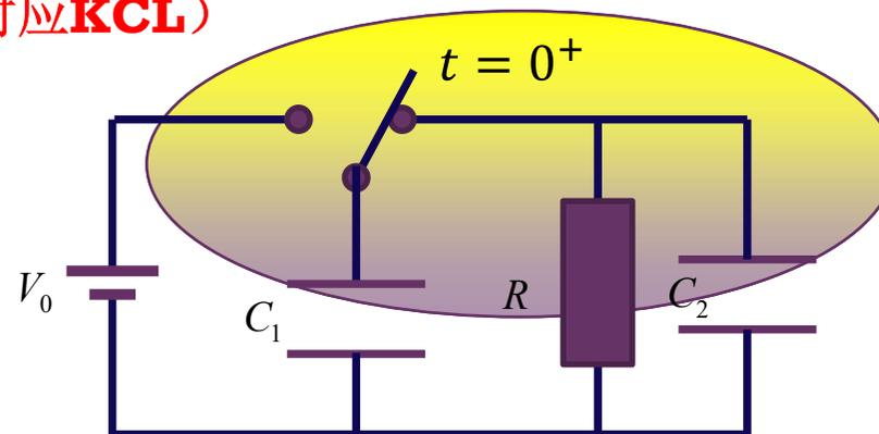
$$v_o(0^+) = \frac{C_1}{C_1 + C_2} V_0$$
