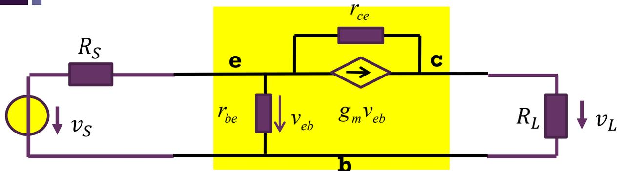
$$\begin{aligned} H = A_v &= \frac{z_{21} R_L}{(z_{22} + R_L)(z_{11} + R_S) - z_{21} z_{12}} \\ &= \frac{(g_m r_{ce} + 1) r_{be} R_L}{(g_m r_{be} r_{ce} + r_{be} + r_{ce} + R_L)(r_{be} + R_S) - r_{be} (g_m r_{ce} + 1) r_{be}} \\ &= \frac{(g_m r_{ce} + 1) r_{be} R_L}{(g_m r_{ce} + 1) r_{be} R_S + (r_{be} + R_S)(r_{ce} + R_L)} \end{aligned}$$
