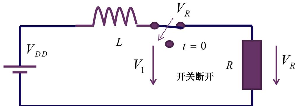
$$i_L(0^-) = \frac{V_{DD}}{R} \quad i_L(0^+) = 0 \quad \text{强行断流}$$
