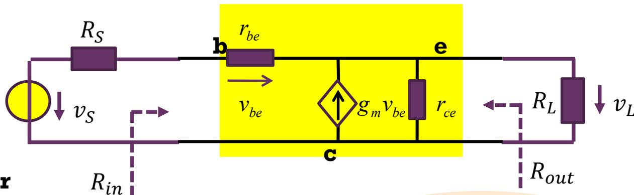
$$R_{in} = g_m r_{be} (r_{ce} \parallel R_L) + r_{be} + r_{ce} \parallel R_L$$
