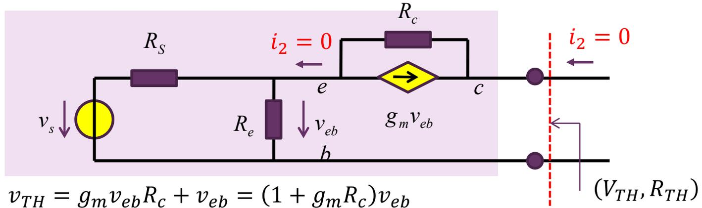
$$= (1 + g_m R_c) \frac{R_e}{R_s + R_e} v_s = (1 + 100m \times 100k) \frac{1k}{0.05k + 1k} v_s = 9525 v_s$$
