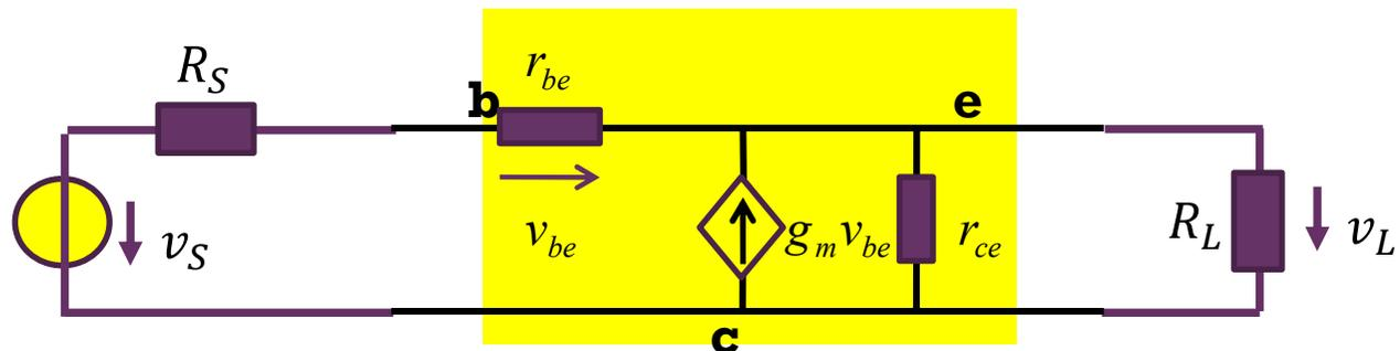
$$\begin{aligned} H = A_v &= \frac{z_{21} R_L}{(z_{22} + R_L)(z_{11} + R_S) - z_{21} z_{12}} \\ &= \frac{(g_m r_{be} + 1) r_{ce} R_L}{(r_{ce} + R_L)(g_m r_{be} r_{ce} + r_{be} + r_{ce} + R_S) - r_{ce} (g_m r_{be} + 1) r_{ce}} \\ &= \frac{(g_m r_{be} + 1) r_{ce} R_L}{(g_m r_{be} + 1) r_{ce} R_L + (r_{be} + R_S)(r_{ce} + R_L)} \end{aligned}$$
