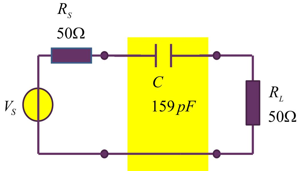
$$C = \frac{\tau}{R_L + R_S} = \frac{1}{2\pi \cdot f_{3dB} \cdot (R_L + R_S)} = \frac{1}{2 \times 3.14 \times 10\text{M} \times (50 + 50)} = 159\text{ pF}$$
