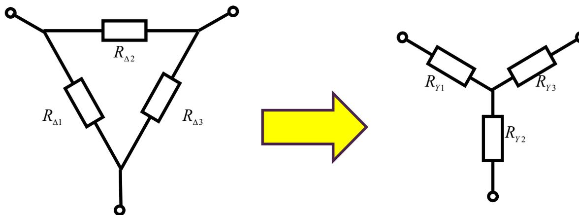
$$R_{Y2} = \frac{G_{\Delta 2}}{G_{\Delta 1}G_{\Delta 3} + G_{\Delta 3}G_{\Delta 2} + G_{\Delta 2}G_{\Delta 1}} = \frac{R_{\Delta 1}R_{\Delta 3}}{R_{\Delta 1} + R_{\Delta 2} + R_{\Delta 3}}$$
