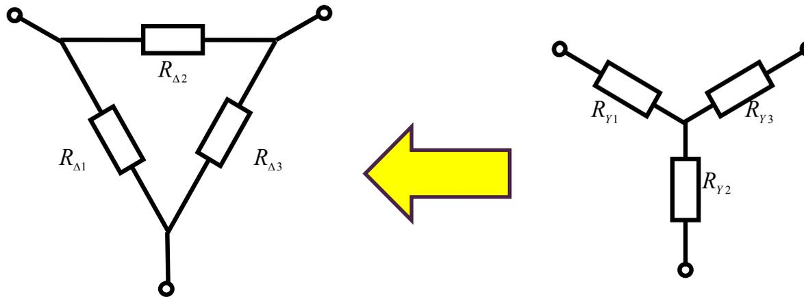
$$R_{\Delta 2} = G_{\Delta 2}^{-1} = \frac{R_{Y1}R_{Y3} + R_{Y3}R_{Y2} + R_{Y2}R_{Y1}}{R_{Y2}} = R_{Y3} + R_{Y1} + \frac{R_{Y1}R_{Y3}}{R_{Y2}}$$
