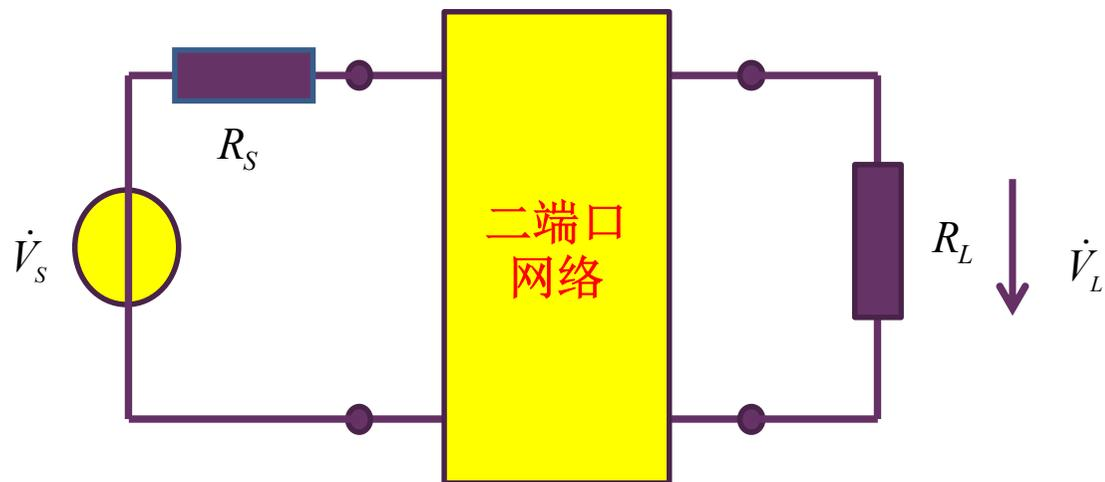
$$|H(j\omega)|^2 = \frac{|\dot{V}_L|^2 / R_L}{|\dot{V}_S|^2 / 4R_S}$$
