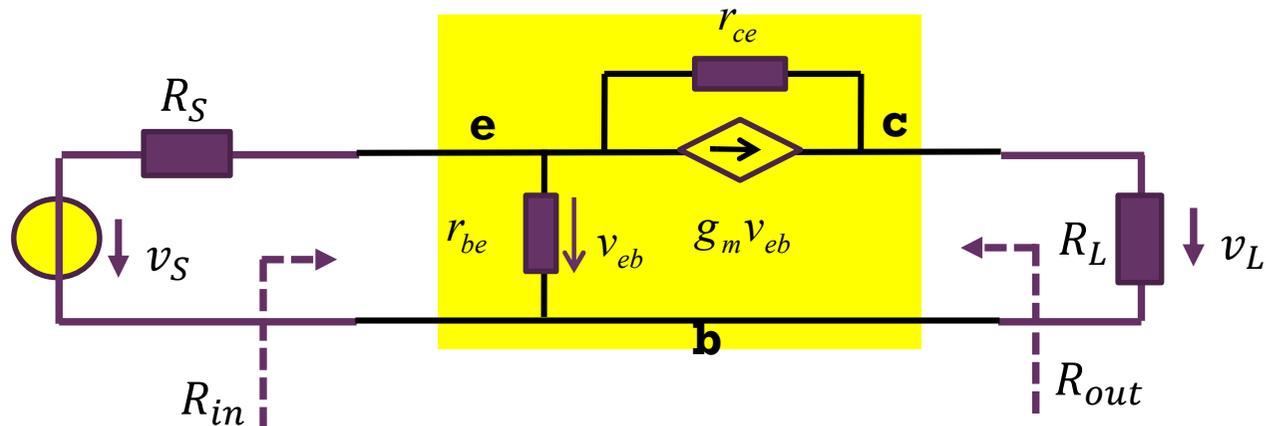
$$R_{in} = r_{be} \parallel \frac{r_{ce} + R_L}{1 + g_m r_{ce}}$$
