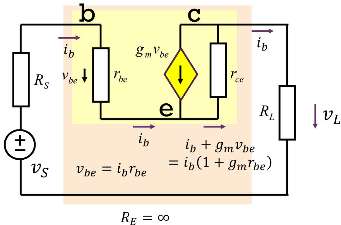
$$R_{in} = r_{be} + \frac{r_{ce} + R_L + g_m r_{be} r_{ce}}{R_E + r_{ce} + R_L} R_E \stackrel{R_E = \infty}{\cong} r_{be} + r_{ce} + R_L + g_m r_{be} r_{ce}$$
