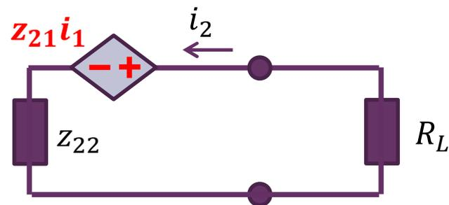
$$v_L = \frac{R_L}{R_L + z_{22}} z_{21} \frac{1}{R_S + z_{11}} v_S$$
