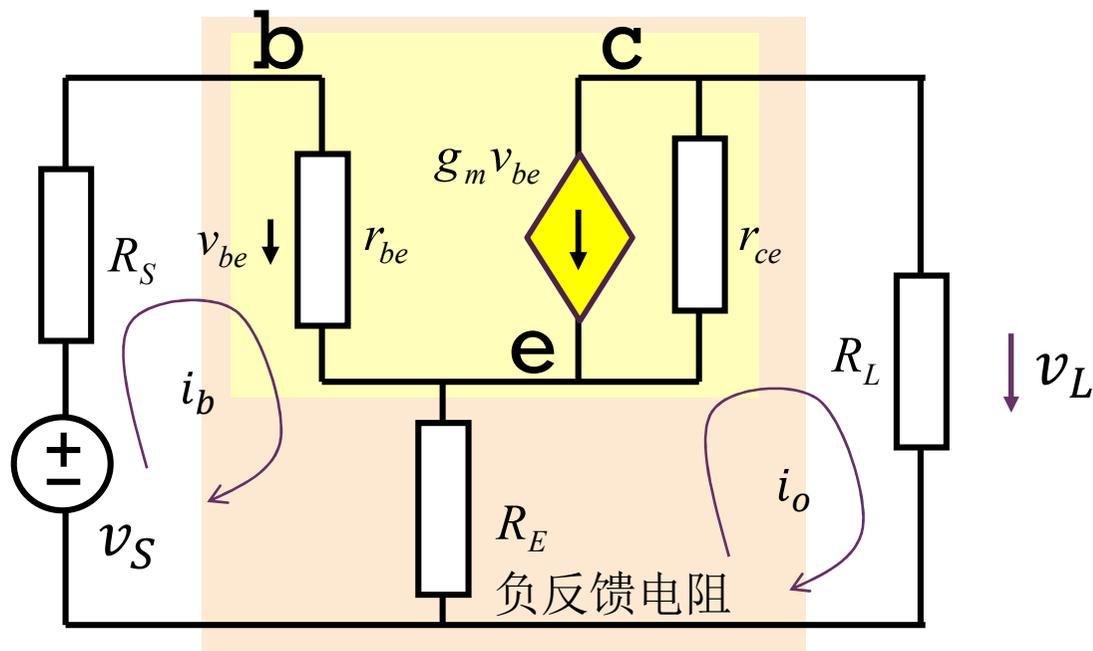
$$\begin{bmatrix} i_b \\ i_o \end{bmatrix} = \frac{\begin{bmatrix} R_E + r_{ce} + R_L \\ R_E - g_m r_{be} r_{ce} \end{bmatrix}}{(R_S + r_{be} + R_E)(R_E + r_{ce} + R_L) + R_E(g_m r_{be} r_{ce} - R_E)} v_S$$
