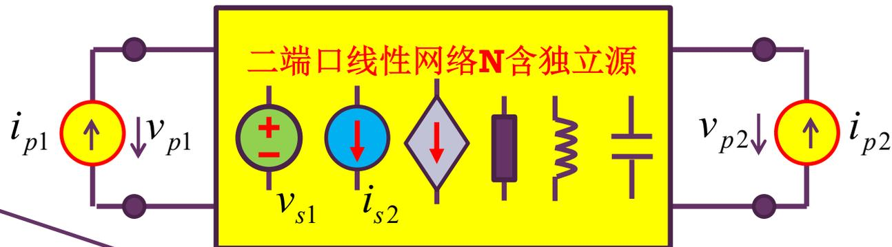
$$v_{p1}(t) = \alpha_{11}i_{p1}(t) + \alpha_{12}i_{p2}(t) + \lambda_{11}v_{s1}(t) + \lambda_{12}i_{s2}(t) + \dots = z_{11}i_{p1}(t) + z_{12}i_{p2}(t) + v_{TH1}(t)$$
