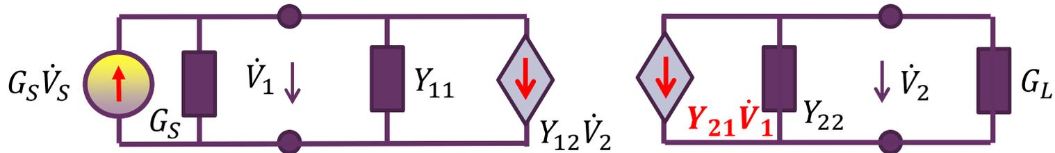
$$\dot{V}_1 = \frac{G_S \dot{V}_S - Y_{12} \dot{V}_2}{G_S + Y_{11}} \quad \dot{V}_2 = -\frac{Y_{21} \dot{V}_1}{G_L + Y_{22}} = -\frac{Y_{21}}{G_L + Y_{22}} \frac{G_S \dot{V}_S - Y_{12} \dot{V}_2}{G_S + Y_{11}}$$
