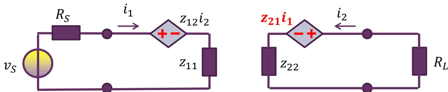
$$i_1 = \frac{v_S - z_{12}i_2}{R_S + z_{11}} \quad i_2 = -\frac{z_{21}i_1}{R_L + z_{22}} = -\frac{z_{21}}{R_L + z_{22}} \frac{v_S - z_{12}i_2}{R_S + z_{11}}$$
