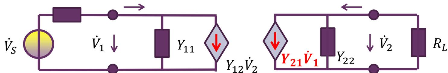
$$H = \frac{\dot{V}_L}{\dot{V}_S} = \frac{\dot{V}_2}{\dot{V}_1} = \frac{Y_{21}G_S}{Y_{21}Y_{12} - (G_S + Y_{11})(G_L + Y_{22})} \stackrel{Y_{12}=0}{=} \frac{-Y_{21}G_S}{(G_S + Y_{11})(G_L + Y_{22})}$$
