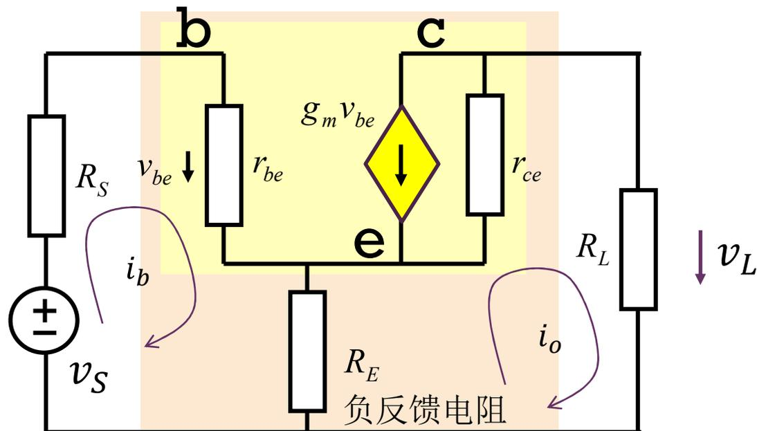
$$\begin{bmatrix} i_b \\ i_o \end{bmatrix} = \frac{\begin{bmatrix} R_E + r_{ce} + R_L \\ R_E - g_m r_{be} r_{ce} \end{bmatrix}}{(R_S + r_{be} + R_E)(R_E + r_{ce} + R_L) + R_E(g_m r_{be} r_{ce} - R_E)} v_S$$
