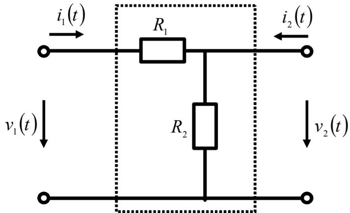
$$v_1 = (R_1 + R_2)i_1 + R_2i_2$$
