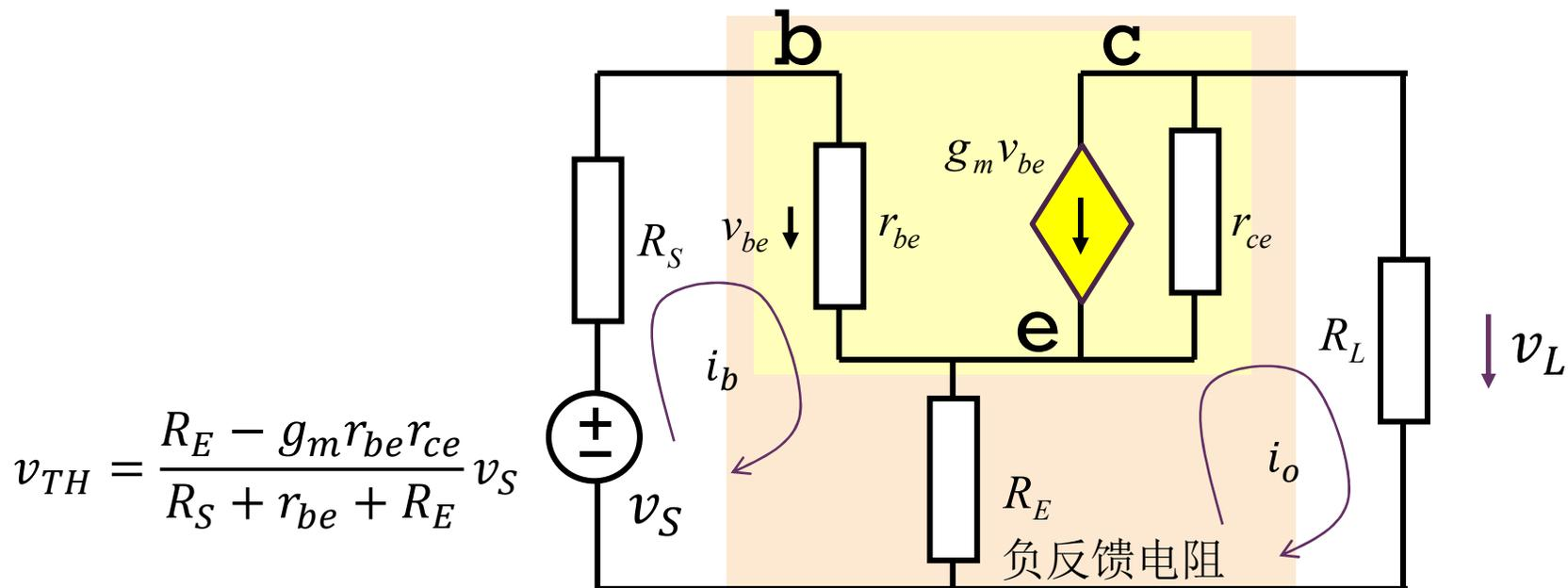
$$v_{TH} = \frac{R_E - g_m r_{be} r_{ce}}{R_S + r_{be} + R_E} v_S$$
