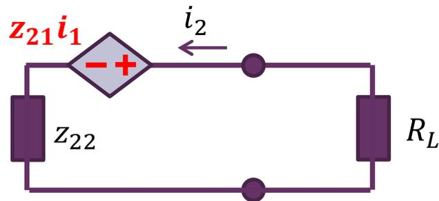
$$A_v = \frac{-z_{21}R_L}{z_{21}z_{12} - (R_L + z_{22})(R_S + z_{11})} \stackrel{z_{12}=0}{=} \frac{z_{21}R_L}{(R_L + z_{22})(R_S + z_{11})}$$
