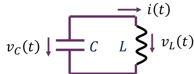
$$\frac{1}{C} \int (-i(t)) dt \stackrel{\text{KCL}}{=} \frac{1}{C} \int i_C(t) dt \stackrel{\text{GOL}}{=} v_C(t) \stackrel{\text{KVL}}{=} v_L(t) \stackrel{\text{GOL}}{=} L \frac{di_L(t)}{dt} \stackrel{\text{KCL}}{=} L \frac{di(t)}{dt}$$
