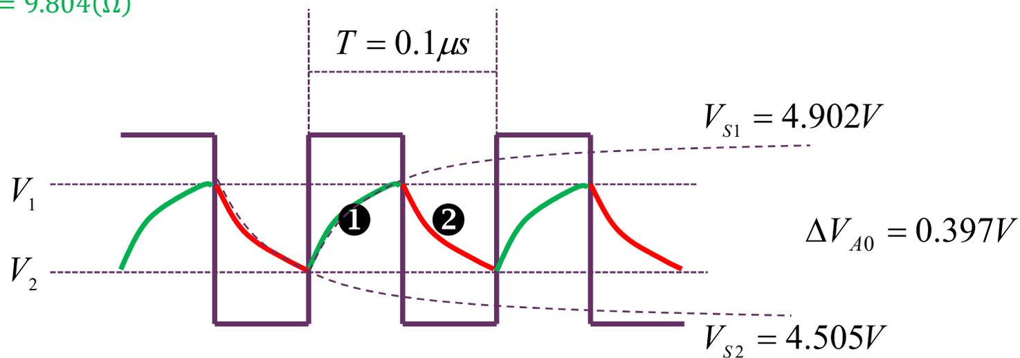
$$\Delta V_A = V_1 - V_2 \leq 0.1\Delta V_{A0} = 0.0397V$$
