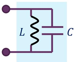
$$\begin{aligned} Y &= Y_C + Y_L = j\omega C + \frac{1}{j\omega L} \\ &= j\left(\omega C - \frac{1}{\omega L}\right) = j\sqrt{\frac{C}{L}}\left(\omega\sqrt{LC} - \frac{1}{\omega\sqrt{LC}}\right) \\ &= jY_0\left(\frac{\omega}{\omega_0} - \frac{\omega_0}{\omega}\right) \stackrel{\omega=\omega_0}{\cong} 0 \end{aligned}$$
