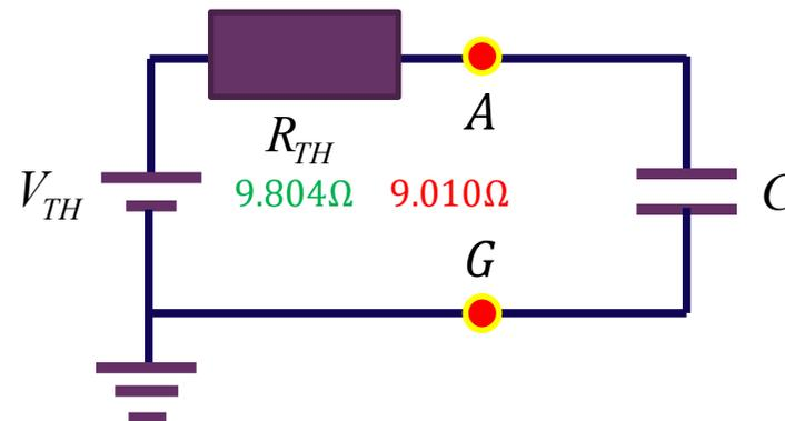
$$\textcircled{1} \quad v_r(t) = V_{S1} + (V_2 - V_{S1})e^{-\frac{\Delta t_1}{\tau_1}} \quad \tau_1 = R_1 C$$
