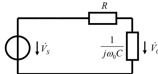
$$\dot{V}_C = \frac{\frac{1}{j\omega_0 C}}{R + \frac{1}{j\omega_0 C}} \dot{V}_S = \frac{1}{1 + j\omega_0 RC} \dot{V}_S$$
