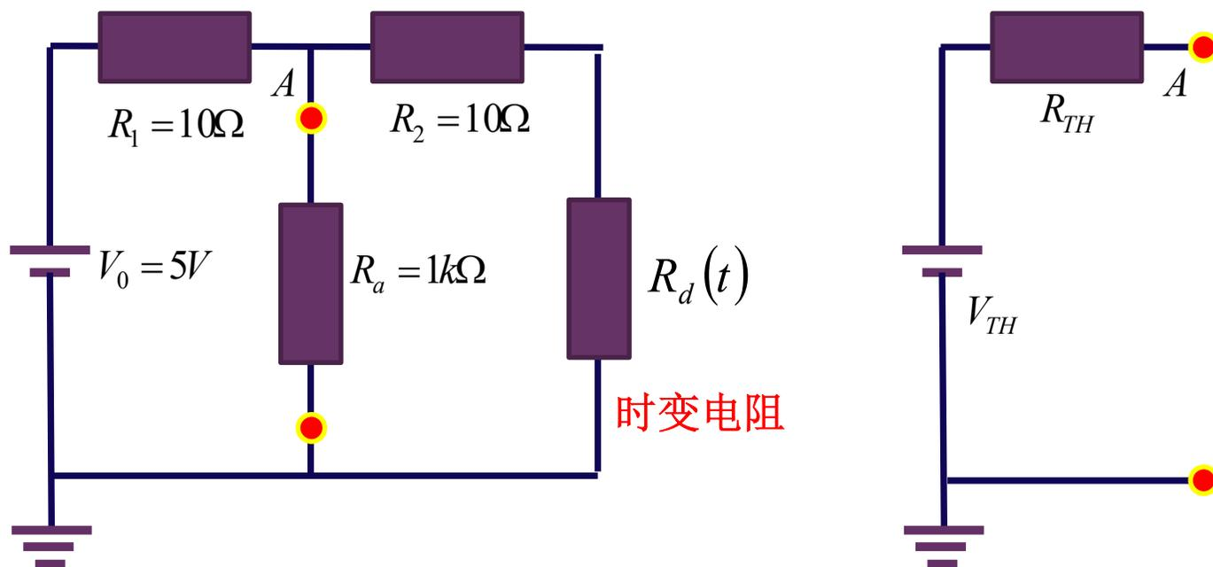
$$R_{TH} = R_1 \parallel R_a \parallel (R_2 + R_d) = \frac{R_a R_1}{R_1 + R_a + \frac{R_a R_1}{R_2 + R_d}}$$
