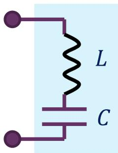
$$\begin{aligned} Z &= Z_L + Z_C = j\omega L + \frac{1}{j\omega C} \\ &= j\left(\omega L - \frac{1}{\omega C}\right) = j\sqrt{\frac{L}{C}}\left(\omega\sqrt{LC} - \frac{1}{\omega\sqrt{LC}}\right) \\ &= jZ_0\left(\frac{\omega}{\omega_0} - \frac{\omega_0}{\omega}\right) \stackrel{\omega=\omega_0}{\cong} 0 \end{aligned}$$
