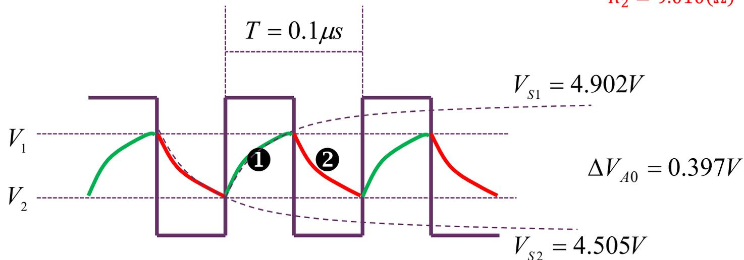
$$\textcircled{1} \quad v_r(t) = V_{S1} + (V_2 - V_{S1})e^{-\frac{\Delta t_1}{\tau_1}}$$
