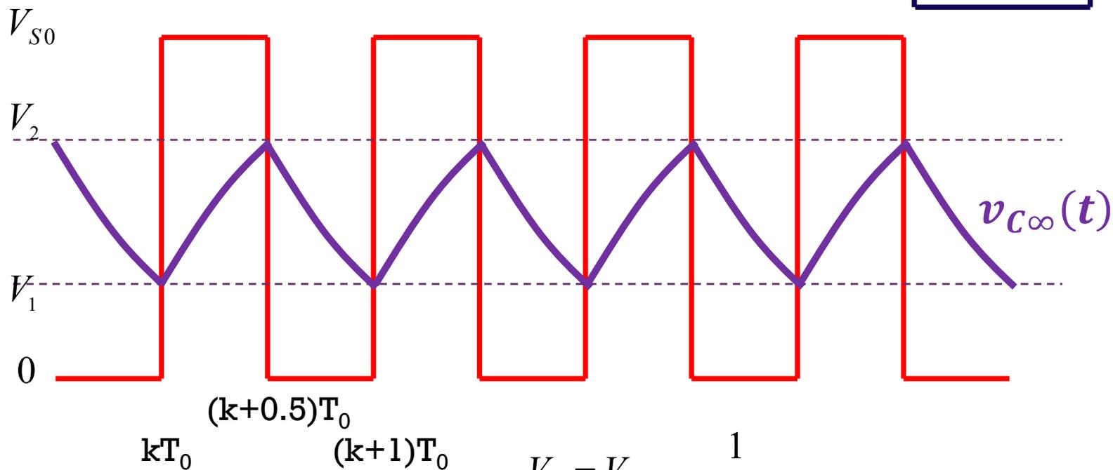
$$V_{S0} + (V_1 - V_{S0})e^{-\frac{0.5T_0}{\tau}} = V_2$$
