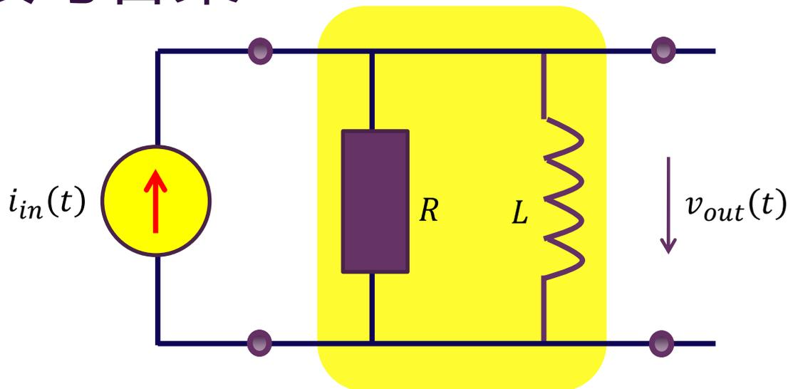
$$H(j\omega) = \frac{\dot{V}_{out}(j\omega)}{\dot{I}_{in}(j\omega)} = H_0 \frac{j\omega\tau}{1 + j\omega\tau}$$
