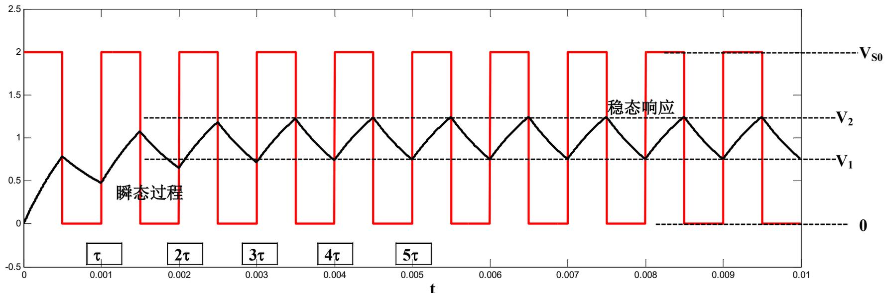
$$v_C(t) = v_{C\infty}(t) + (v_C(0^+) - v_{C\infty}(0^+))e^{-\frac{t}{\tau}} = v_{C\infty}(t) - V_{S0} \frac{e^{-\frac{t}{\tau}}}{1 + e^{\frac{0.5T_0}{\tau}}}$$
