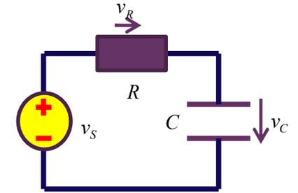
$$kT_0 \sim (k + 0.5)T_0 : \quad v_{C\infty}(t) = V_{S0} \left[ 1 - \frac{1}{1 + e^{-\frac{0.5T_0}{\tau}}} e^{-\frac{t-kT_0}{\tau}} \right]$$
