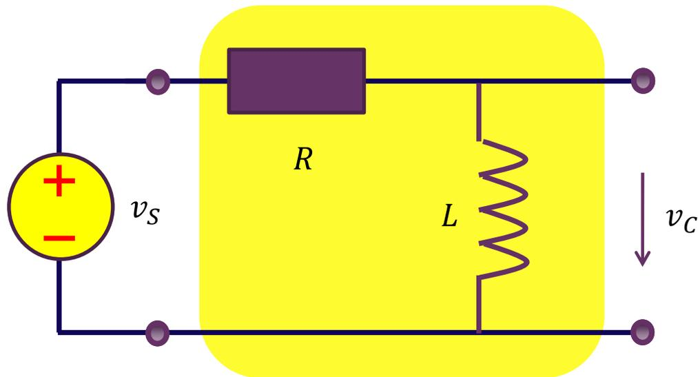
$$H_{v_L} = \frac{j\omega L}{R + j\omega L} = \frac{j\omega GL}{1 + j\omega GL}$$
