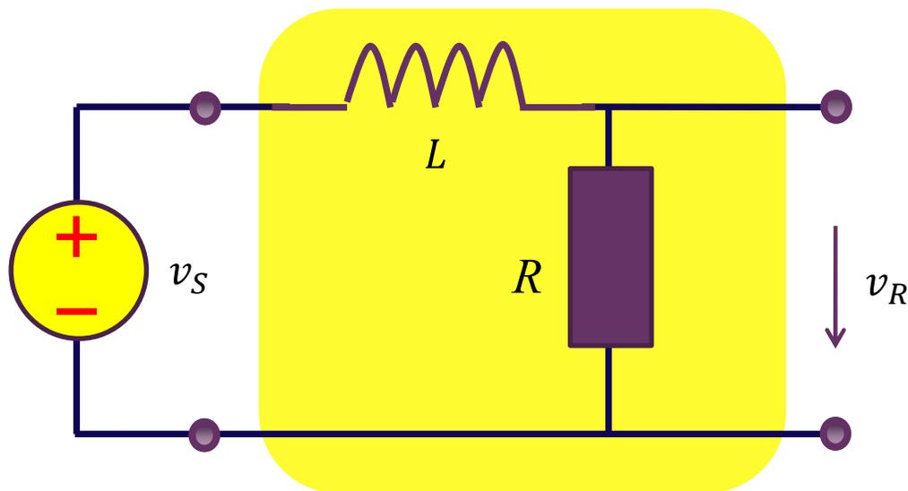
$$H_{v_R} = \frac{R}{R + j\omega L} = \frac{1}{1 + j\omega GL}$$
