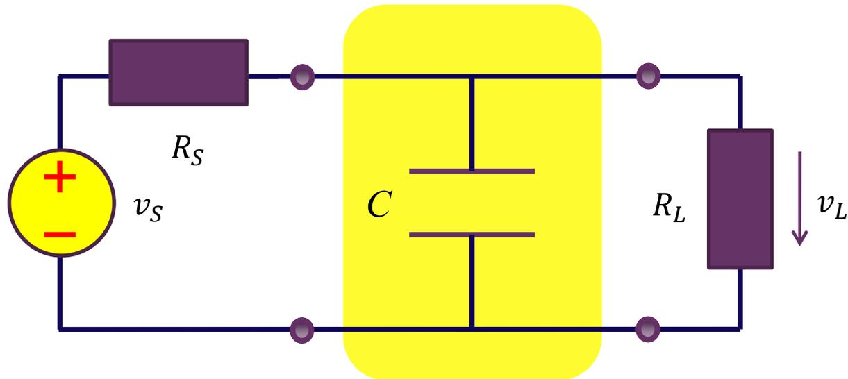
$$H(j\omega) = 2 \sqrt{\frac{R_S \dot{V}_L(j\omega)}{R_L \dot{V}_S(j\omega)}} = 2 \sqrt{\frac{R_S}{R_L} \frac{R_L}{R_S + R_L} \frac{1}{1 + j\omega \frac{R_S R_L}{R_S + R_L} C}} = H_0 \frac{1}{1 + j\omega\tau}$$
