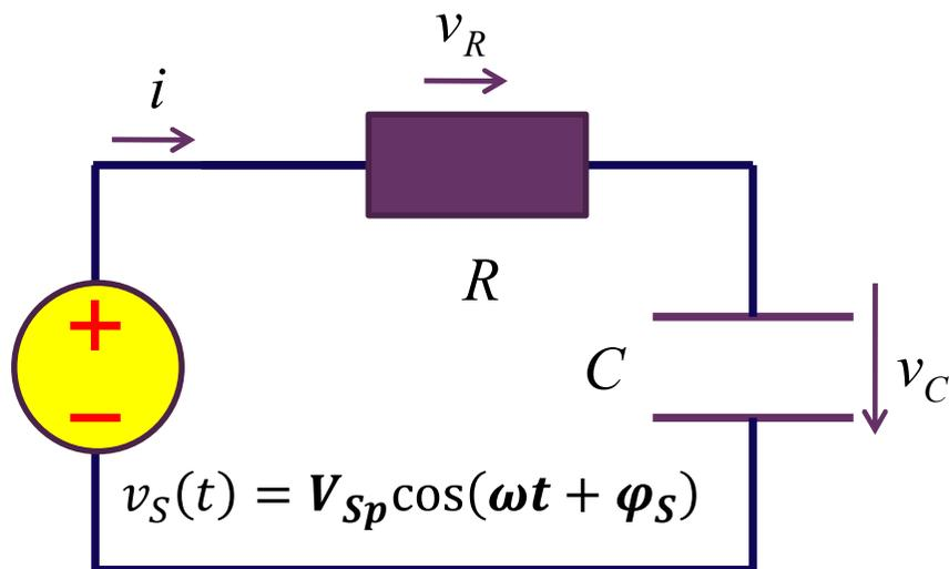
$$v_R(t) = \frac{\omega RC}{\sqrt{1 + (\omega RC)^2}} V_{Sp} \cos\left(\omega t + \varphi_S + \frac{\pi}{2} - \arctan \omega RC\right)$$
