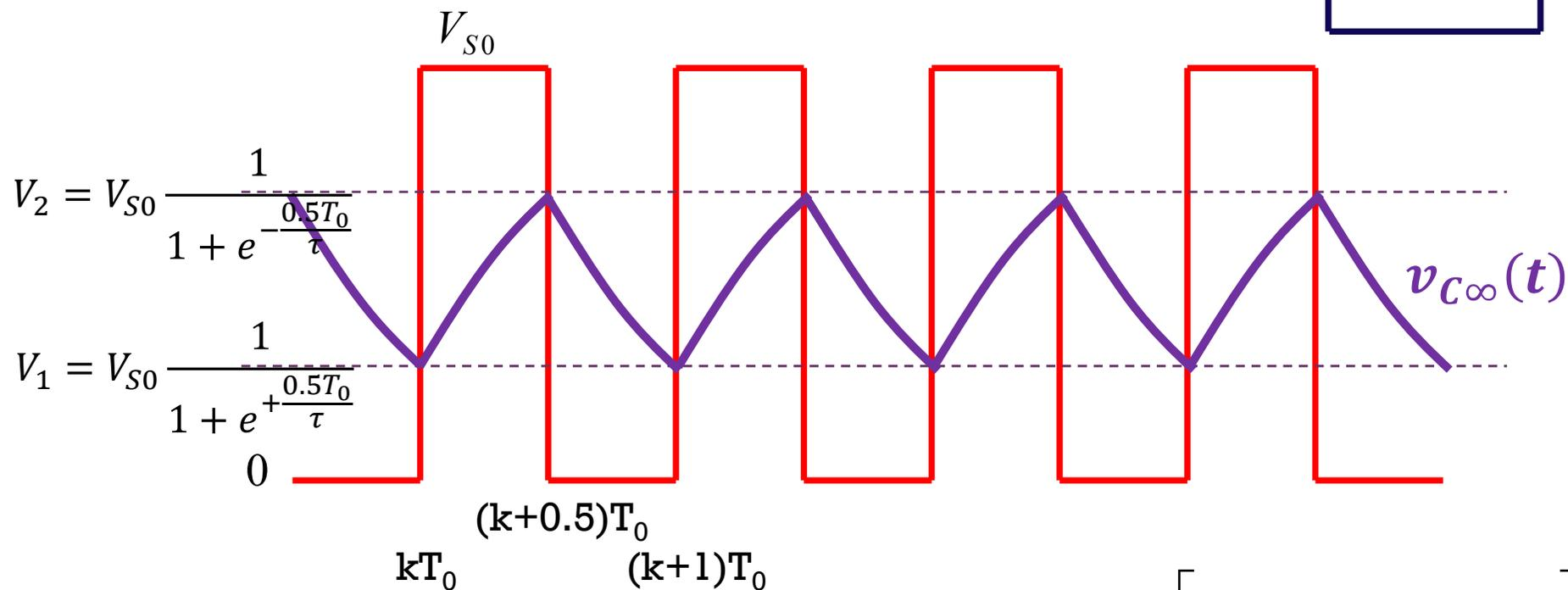
$$kT_0 \sim (k+0.5)T_0: \quad v_{C\infty}(t) = V_{S0} + (V_1 - V_{S0})e^{-\frac{t-kT_0}{\tau}} = V_{S0} \left[ 1 - \frac{1}{1 + e^{-\frac{0.5T_0}{\tau}}} e^{-\frac{t-kT_0}{\tau}} \right]$$
