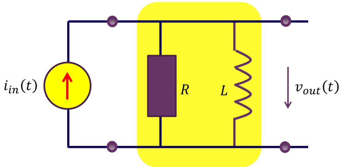
$$H(j\omega) = \frac{\dot{V}_{out}(j\omega)}{\dot{I}_{in}(j\omega)} = R_{m0}(j\omega) = \frac{R \times j\omega L}{R + j\omega L} = R \frac{j\omega GL}{1 + j\omega GL} = R \frac{j\omega\tau}{1 + j\omega\tau} = H_0 \frac{j\omega\tau}{1 + j\omega\tau}$$
