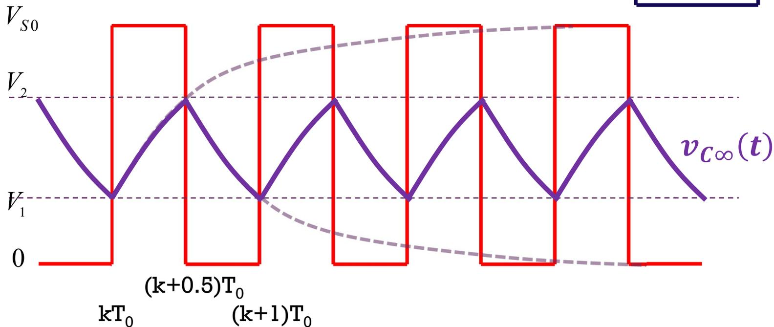
$$kT_0 \sim (k+0.5)T_0: \quad v_{C\infty}(t) = V_{S0} + (V_1 - V_{S0})e^{-\frac{t-kT_0}{\tau}} \quad V_{S0} + (V_1 - V_{S0})e^{-\frac{0.5T_0}{\tau}} = V_2$$
