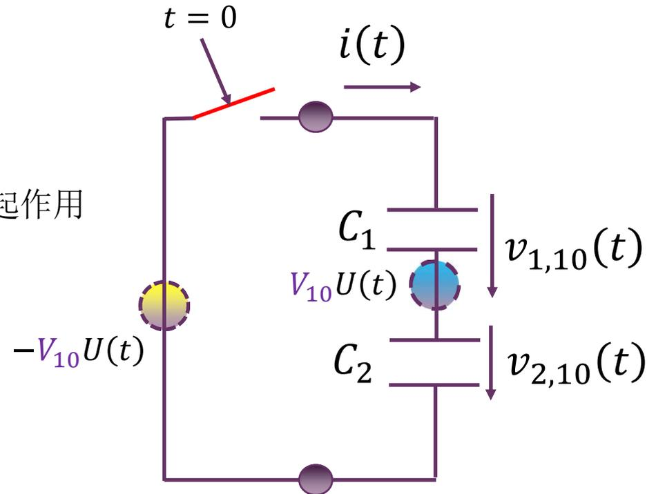
$$v_{1,10}(t) = -\frac{C_2}{C_1 + C_2} V_{10}U(t) + V_{10}U(t)$$
