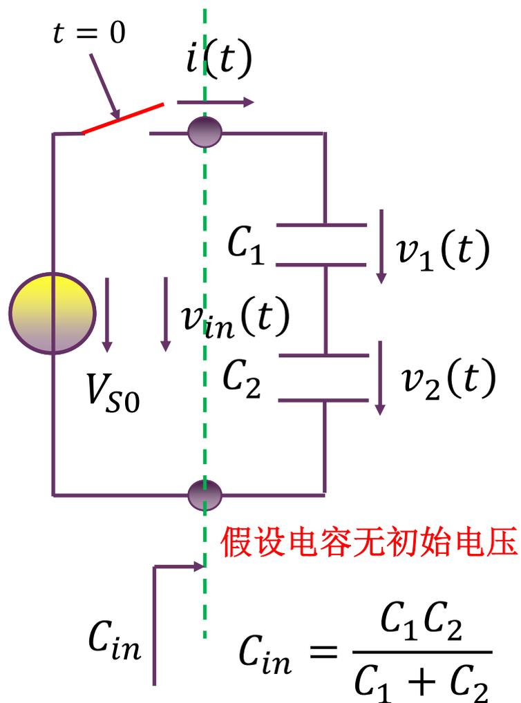
$$v_{in}(t) = V_{S0} U(t)$$
