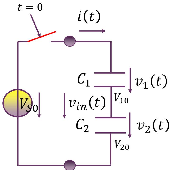
$$v_1(t) = v_{1,s0}(t) + v_{1,10}(t) + v_{1,20}(t)$$
