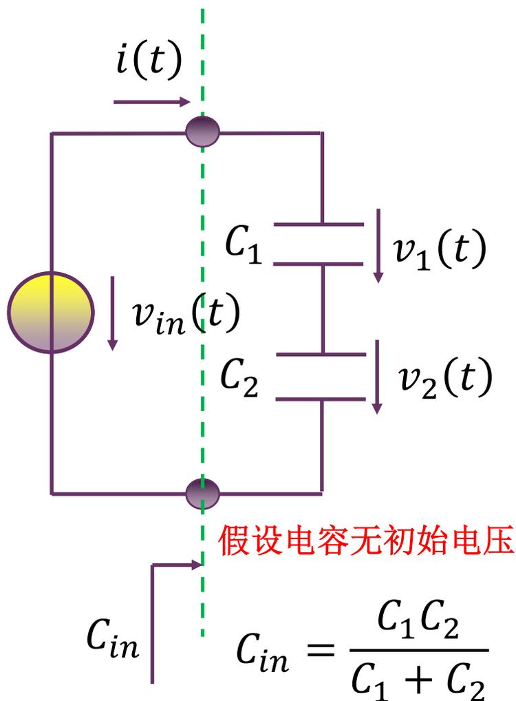
$$i(t) = C_{in} \frac{d}{dt} v_{in}(t)$$
