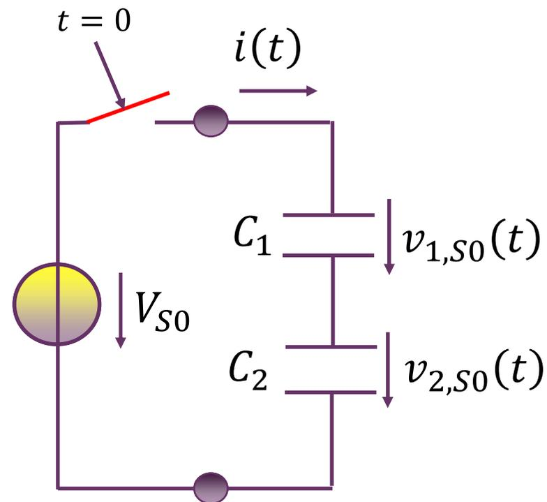
$$v_{1,S0}(t) = \frac{C_2}{C_1 + C_2} V_{S0} U(t)$$
