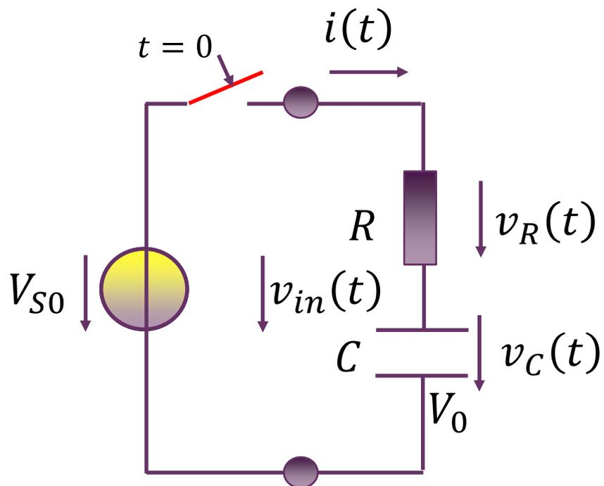
$$v_R(t) = (V_{S0} - V_0)e^{-\frac{t}{\tau}}U(t)$$
