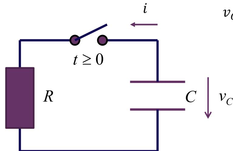
$$v_C(t) = \frac{1}{C} \int_{-\infty}^t i_C(t) dt = V_0 + \frac{1}{C} \int_0^t i_C(t) dt$$
