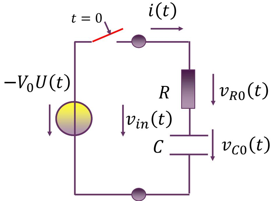
$$v_C(t) = v_{C0}(t) + V_0 U(t)$$
