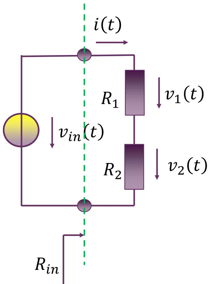
$$R_{in} = R_1 + R_2$$
