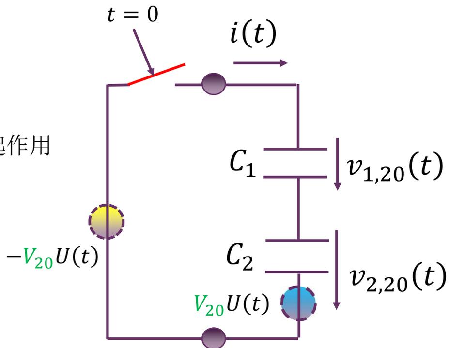
$$v_{1,20}(t) = -\frac{C_2}{C_1 + C_2} V_{20}U(t)$$
