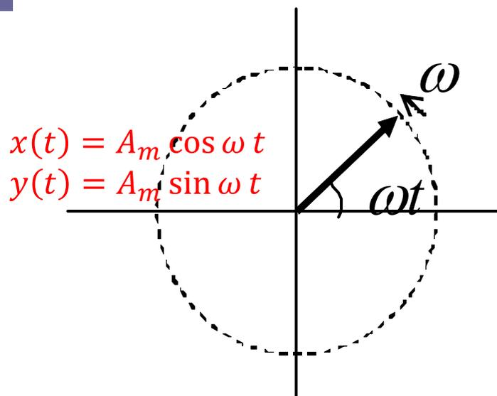
$$\begin{aligned}\vec{s}(t) &= x(t)\hat{x} + y(t)\hat{y} \\ s(t) &= x(t) + jy(t) \\ &= A_m \cos \omega t + jA_m \sin \omega t \\ &= A_m e^{j\omega t} = s_+\end{aligned}$$
