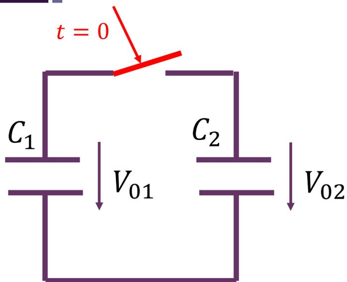
$$v_2(0^+) = v_1(0^+) = \frac{C_1 V_{01} + C_2 V_{02}}{C_1 + C_2}$$
