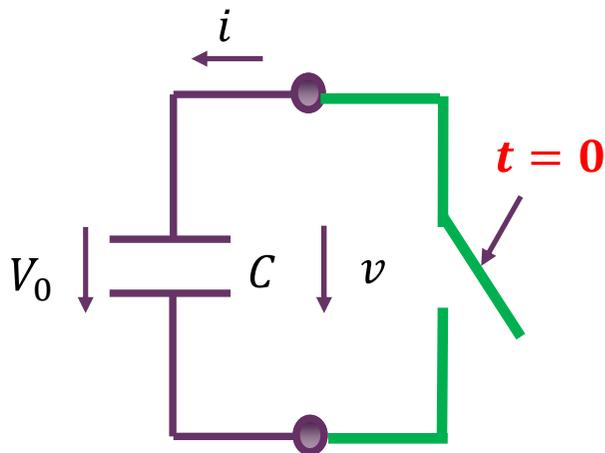
$$v_C(0^-) = V_0 \quad E_C(0^-) = \frac{1}{2} CV_0^2$$
