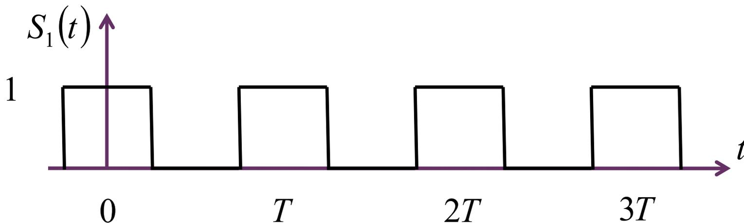
$$S_1(t) = \frac{1}{2} + \frac{2}{\pi} \cos \omega_0 t - \frac{2}{3\pi} \cos 3\omega_0 t + \frac{2}{5\pi} \cos 5\omega_0 t - \dots$$
