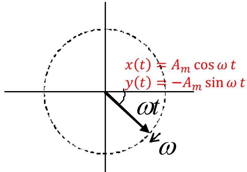
$$\begin{aligned}\vec{s}(t) &= x(t)\hat{x} + y(t)\hat{y} \\ s(t) &= x(t) + jy(t) \\ &= A_m \cos \omega t - jA_m \sin \omega t \\ &= A_m \cos(-\omega t) + jA_m \sin(-\omega t) \\ &= A_m e^{-j\omega t} = s_-\end{aligned}$$
