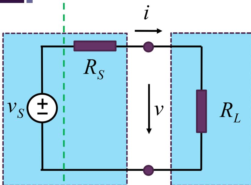
$$v = iR_L = \frac{R_L}{R_S + R_L} v_S$$
