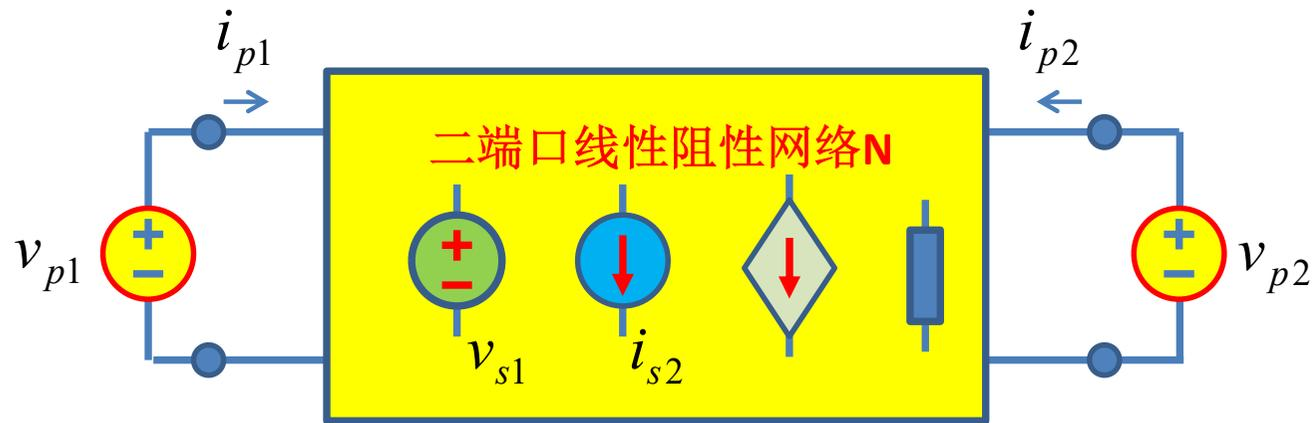
$$i_{p1} = \alpha_{11}v_{p1} + \alpha_{12}v_{p2} + \lambda_{11}v_{s1} + \lambda_{12}i_{s2} + \dots = G_{11}v_{p1} + G_{12}v_{p2} + i_{N1}$$
