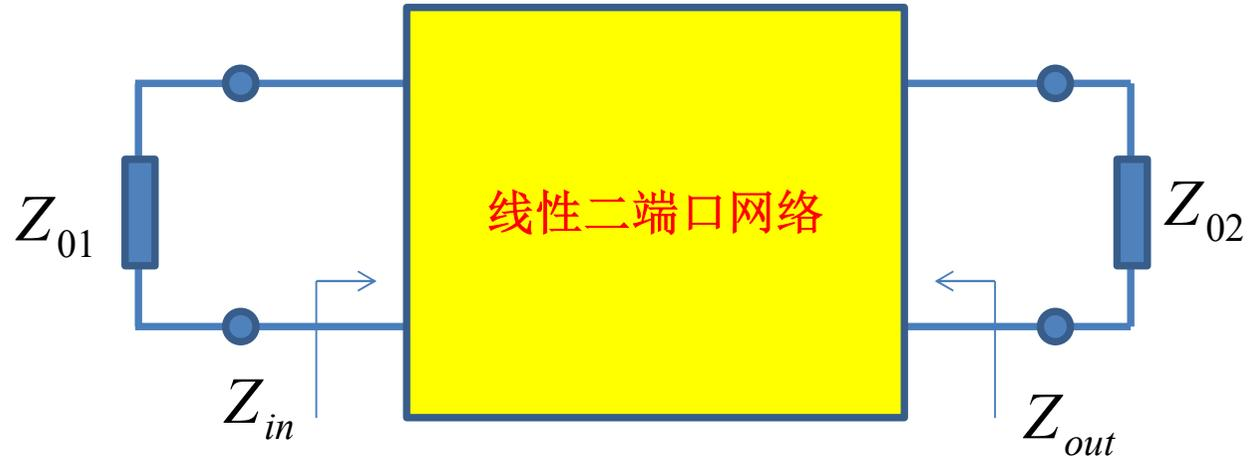
$$Z_{01} = Z_{in} = z_{11} - \frac{z_{12}z_{21}}{z_{22} + Z_{02}} \quad Z_{02} = Z_{out} = z_{22} - \frac{z_{21}z_{12}}{z_{11} + Z_{01}}$$
