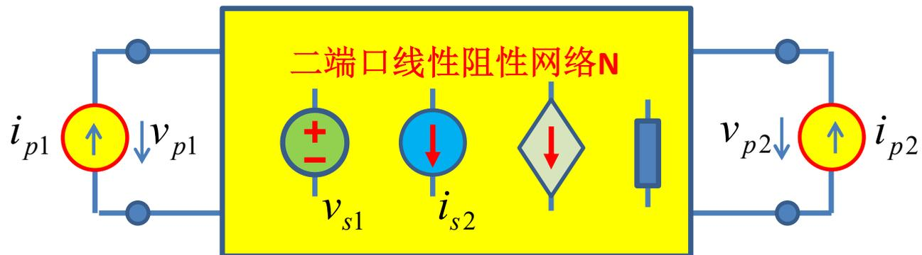
$$v_{p1} = \alpha_{11}i_{p1} + \alpha_{12}i_{p2} + \lambda_{11}v_{s1} + \lambda_{12}i_{s2} + \dots = R_{11}i_{p1} + R_{12}i_{p2} + v_{TH1}$$
