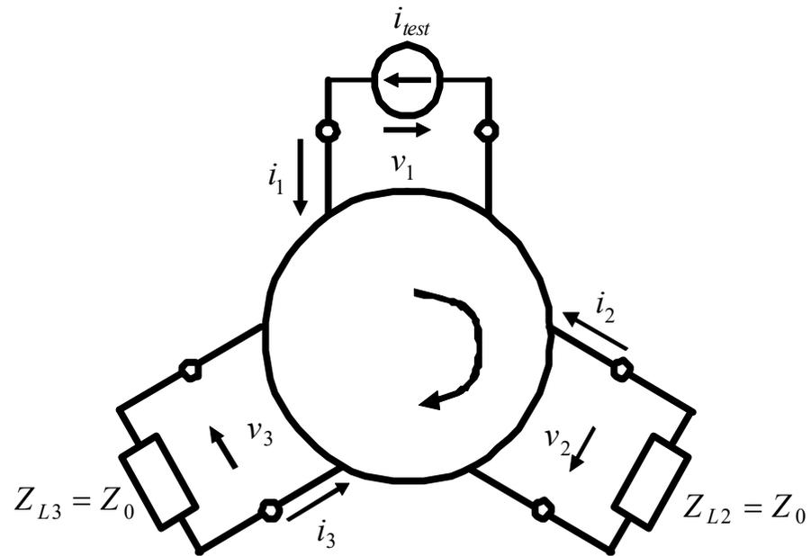
$$v_{test} = \frac{2Z_0 R^2}{Z_0^2 + R^2} i_{test}$$
