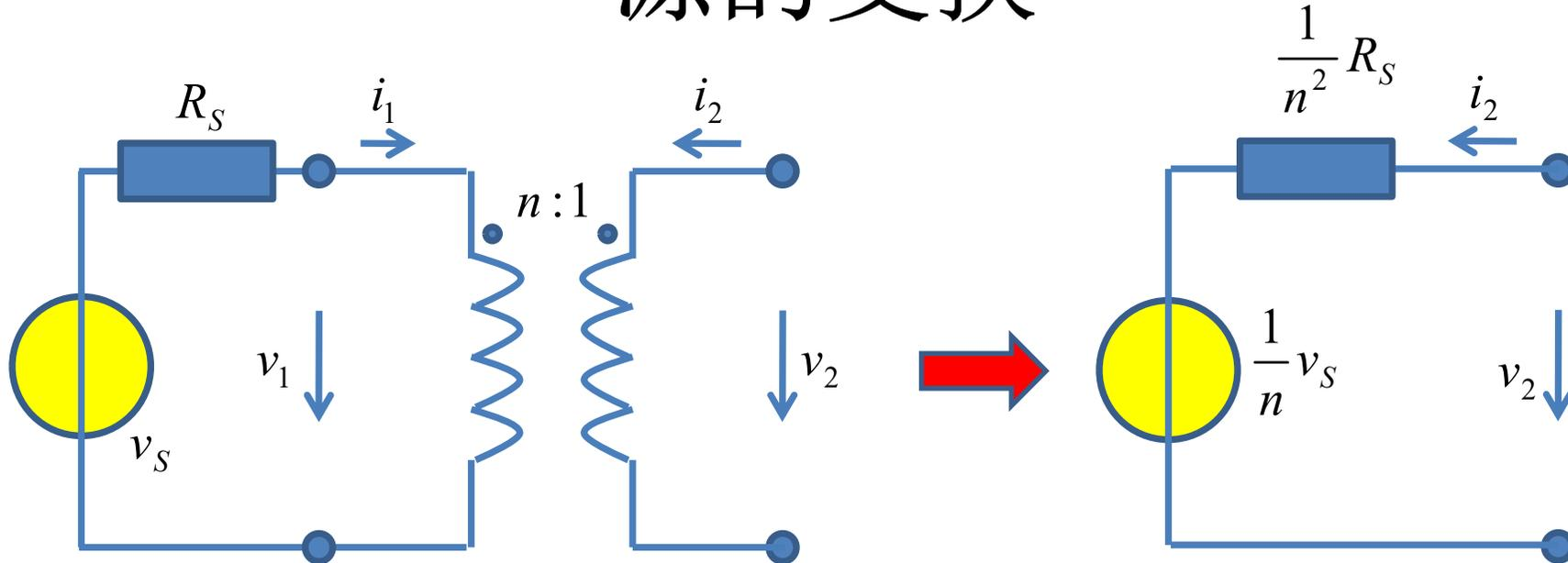
$$v_1 = nv_2; \quad i_1 = -\frac{1}{n}i_2$$
