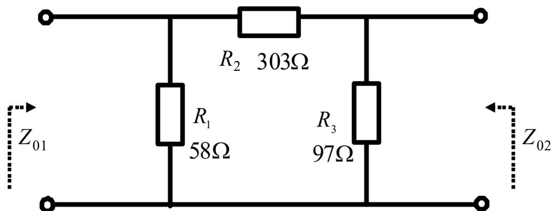
$$Z_{01} = \sqrt{(R_1 \parallel R_2) \cdot (R_1 \parallel (R_2 + R_3))} = \sqrt{(58 \parallel 303) \cdot (58 \parallel (303 + 97))} = 49.7\Omega \approx 50\Omega$$
