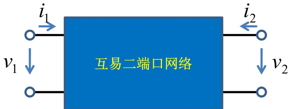
$$\frac{-i_{2,short}}{v_{s1}} = -y_{21} = -y_{12} = \frac{-i_{1,short}}{v_{s2}}$$
