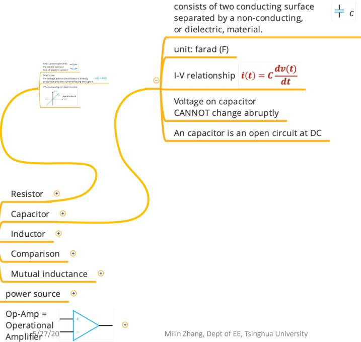
A CAPACITOR is a circuit element that
