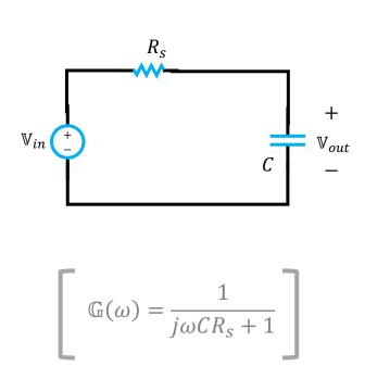
This is a LOW PASS FILTER Which passes low frequencies and block high frequencies
