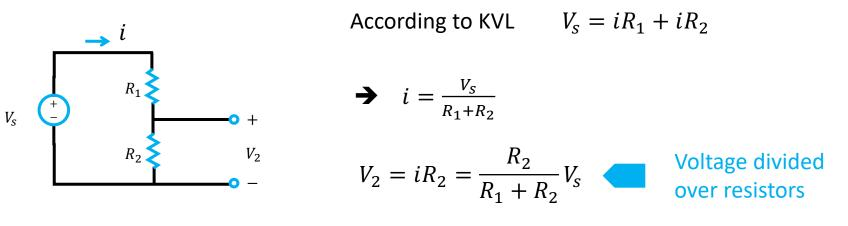
**QUESTION:** calculate the voltage transfers from input to output based on varying  $R_2$
