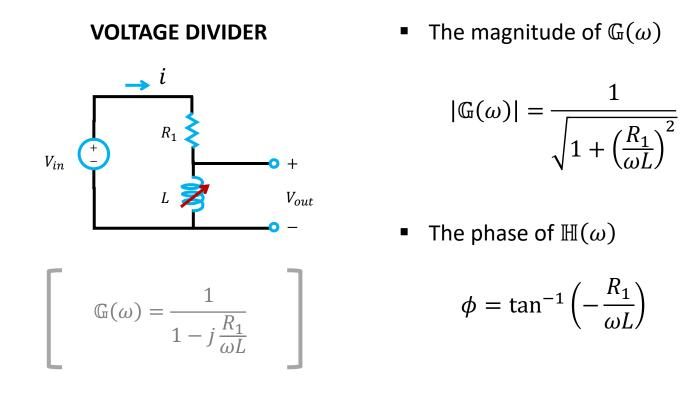
**QUESTION:** calculate the voltage transfers from input to output based on varying L
