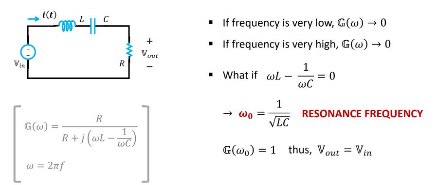
The RESONANCE FREQUENCY,  $\omega_0$ , at which the impedance of the circuit is purely real. The circuit itself at  $\omega_0$  is called IN RESONANCE.
