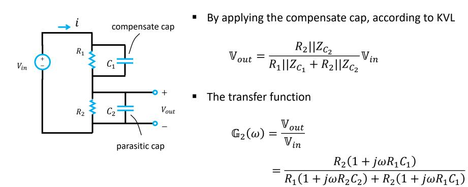
**QUESTION:** a voltage divider usually does work well at high frequency due to the parasitic capacitance. In order to remedy this capacitance issue, a small capacitor in parallel with the series resistor is applied. This capacitor is called compensate capacitor. Find the proper value of the compensate capacitor.
