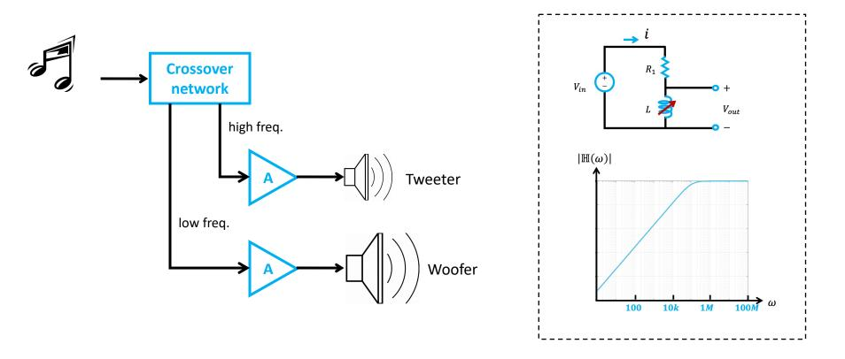
**QUESTION:** design a stereo amplifier with two output channels to split the high and low frequencies.
