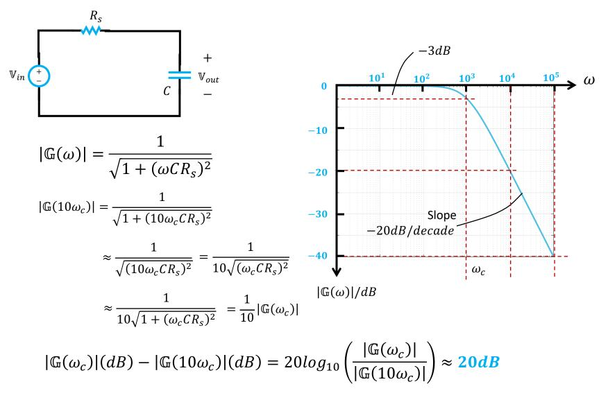
**BODE PLOT generates a "straight-line" approximation of the transfer function**
