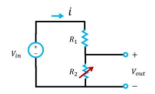
$$V_{out} = iR_2 = \frac{R_2}{R_1 + R_2} V_{in}$$
