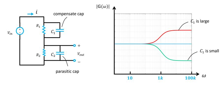
$$\mathbb{G}_{2}(\omega) = \frac{R_{2}(1+j\omega R_{1}C_{1})}{R_{1}(1+j\omega R_{2}C_{2})+R_{2}(1+j\omega R_{1}C_{1})}$$
