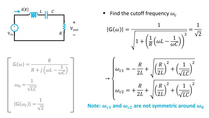
**QUESTION:** calculate the voltage transfers from input to output based on varying *R*
