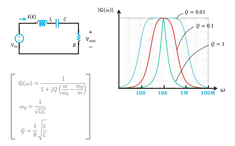
**QUESTION:** calculate the voltage transfers from input to output based on varying *R*
