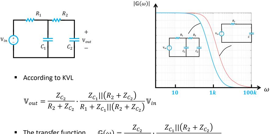
• The transfer function  $\mathbb{G}(\omega) = \frac{Z_{C_2}}{R_2 + Z_{C_2}} \cdot \frac{Z_{C_1}||(R_2 + Z_{C_2})}{R_1 + Z_{C_1}||(R_2 + Z_{C_2})}$
