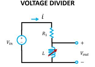
$$\mathbb{G}(R_2) = \frac{\mathbb{V}_{out}}{\mathbb{V}_{in}} = \frac{j\omega L}{R_1 + j\omega L} = \frac{1}{\frac{R_1}{j\omega L} + 1}$$
