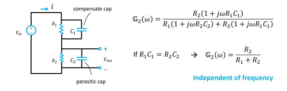
**QUESTION:** a voltage divider usually does work well at high frequency due to the parasitic capacitance. In order to remedy this capacitance issue, a small capacitor in parallel with the series resistor is applied. This capacitor is called compensate capacitor. Find the proper value of the compensate capacitor.
