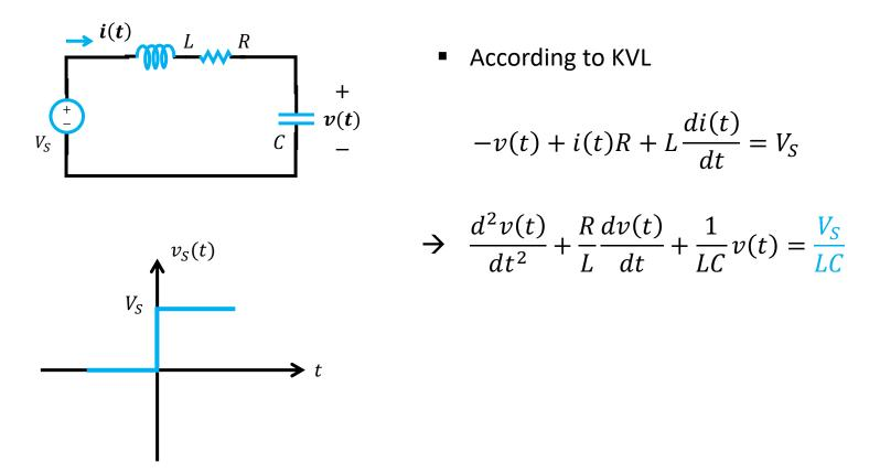
**QUESTION:** Find how the voltage on the capacitor and the current through the inductor change with an input voltage of step function.
