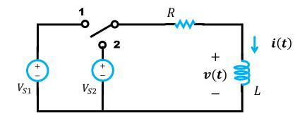
When the switch turned to node 1, according to KVL
