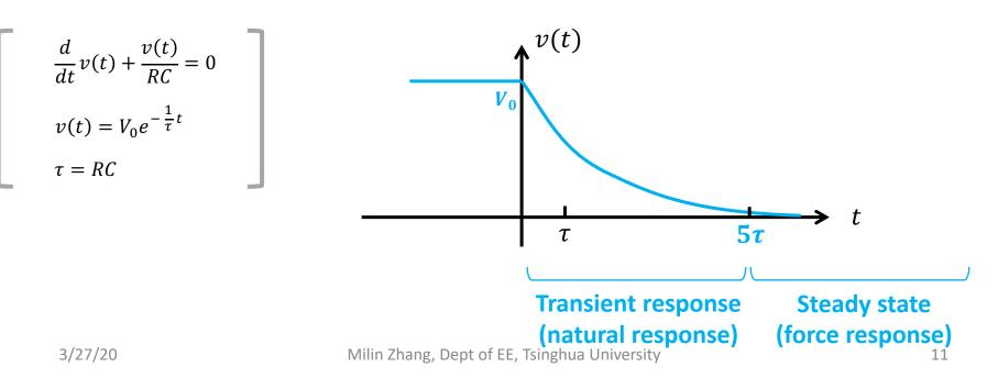
**QUESTION:** Assume the capacitor C has been charged to  $V_0$  before the switch is turned on. Find the response after the switch is turned on.
