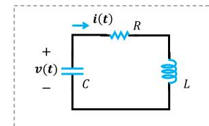
Series connected RLC circuit
