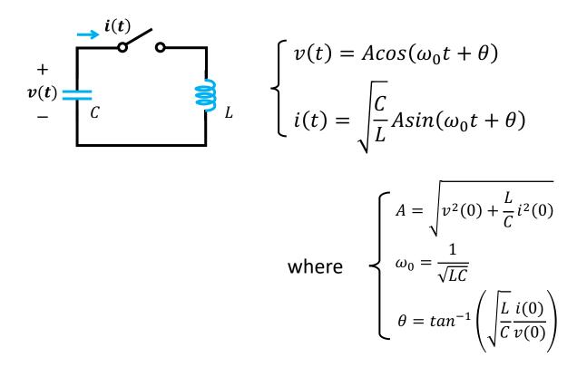
**QUESTION:** Find how the voltage on the capacitor and the current through the inductor change after the switch is turned on.
