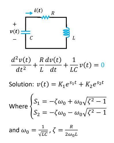
**QUESTION:** Find how the voltage on the capacitor and the current through the inductor change with an input voltage of step function.
