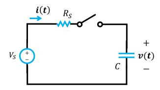
$$\frac{d}{dt}v(t) + \frac{1}{RC}v(t) = \frac{1}{RC}V_S$$
