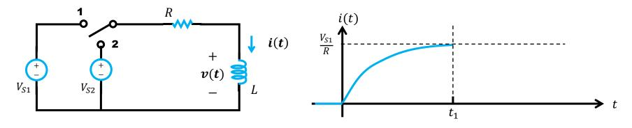
• The full solution  $i(t) = i_p(t) + i_c(t) = \frac{V_{S1}}{R} + K_2 e^{-\frac{R}{L}t}$
