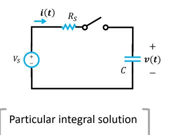
$$\frac{d}{dt}v(t) + \frac{1}{RC}v(t) = \frac{1}{RC}V_S$$
