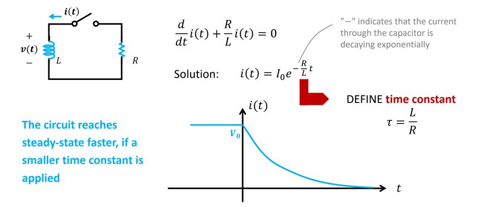
**QUESTION:** Assume the capacitor L has been charged to  $I_0$  before the switch is turned on. Find the response after the switch is turned on.
