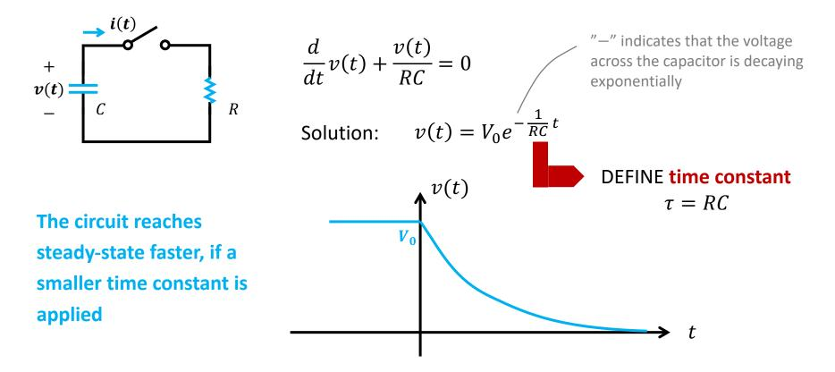
**QUESTION:** Assume the capacitor C has been charged to  $V_0$  before the switch is turned on. Find the response after the switch is turned on.
