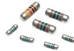
Metal Electrode Leadless Face (MELF) resistor
