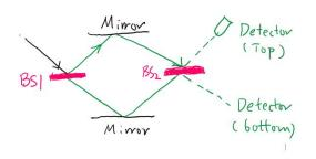
For the Mach-Zehnder interference setup to detect the F-V bomb, we know that BS1, BS2 are identical R=50%-T=50% beam splitters. In terms of reflection and transmission coefficients:
