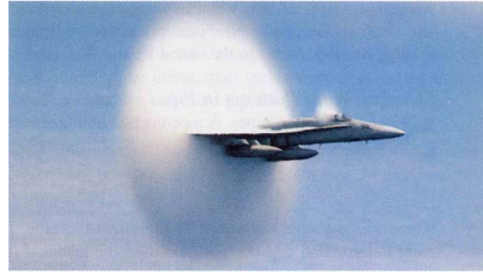
Fig. 18-24 Shock waves produced by the wings of a Navy FA 18 jet. They are visible because the sudden decrease in air pressure in the shock waves caused water molecules in the air to condense, forming a fog.
