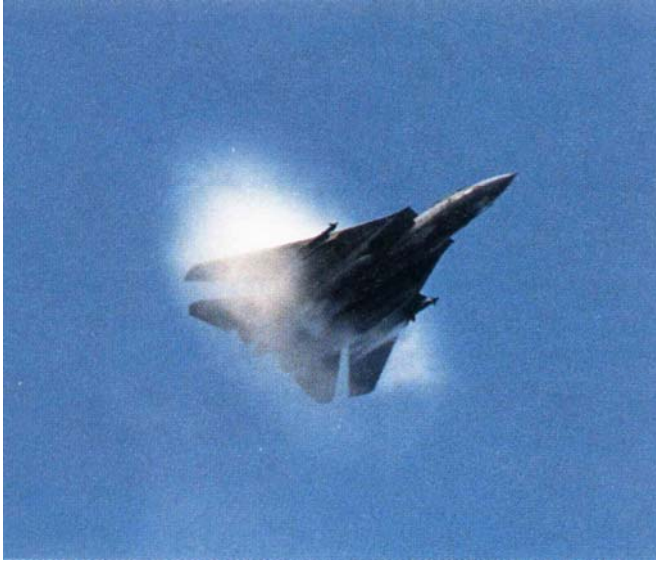
Fig. 18-24 Shock waves produced by the wings of a Navy FA 18 jet. They are visible because the sudden decrease in air pressure in the shock waves caused water molecules in the air to condense, forming a fog.
