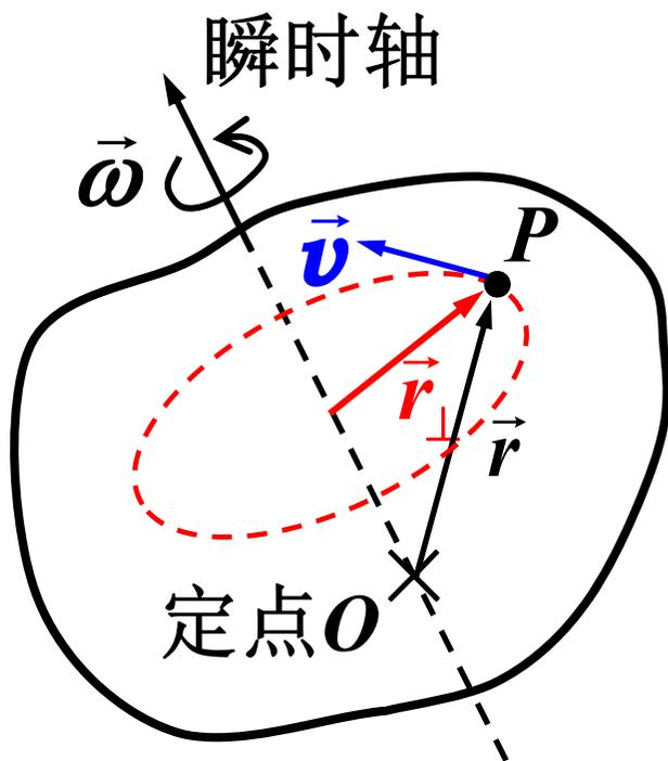
$$\vec{v} = \vec{\omega} \times \vec{r}_{\perp} = \vec{\omega} \times \vec{r}$$
