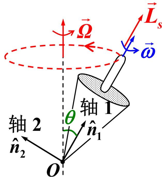
$$\vec{\omega}_{\text{总}} = \vec{\omega} + \vec{\Omega} = (\omega + \Omega \cos \theta) \cdot \hat{n}_1 + \Omega \sin \theta \cdot \hat{n}_2$$
