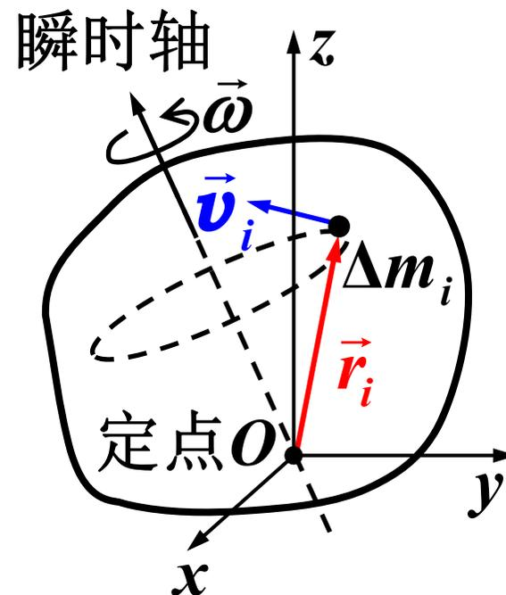
$$E_k = \frac{1}{2} (\omega_x \quad \omega_y \quad \omega_z) \begin{bmatrix} J_{xx} & J_{xy} & J_{xz} \\ J_{yx} & J_{yy} & J_{yz} \\ J_{zx} & J_{zy} & J_{zz} \end{bmatrix} \begin{pmatrix} \omega_x \\ \omega_y \\ \omega_z \end{pmatrix}$$
