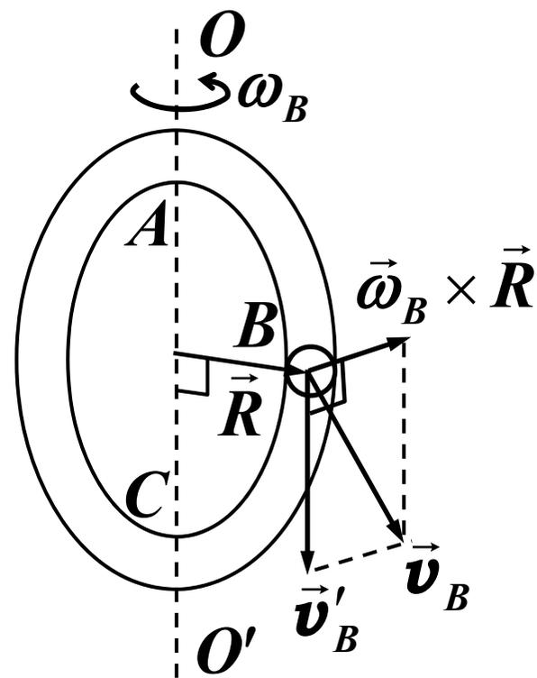
$$\begin{aligned} A \rightarrow B: \quad \frac{1}{2} J \omega_0^2 + mgR &= \frac{1}{2} J \omega_B^2 + \frac{1}{2} m v_B^2 \\ &= \frac{1}{2} J \omega_B^2 + \frac{1}{2} m (v_B'^2 + \omega_B^2 R^2) \end{aligned}$$
