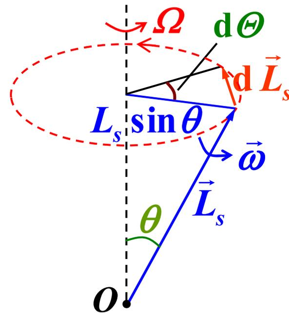
或者:  $\frac{d\vec{L}_s}{dt} = \vec{\Omega} \times \vec{L}_s = \vec{M} \Rightarrow \Omega L_s \sin\theta = M$
