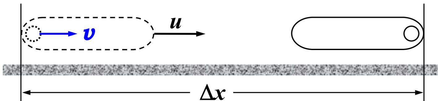
$$\left. \begin{aligned} \Delta x &= \gamma(\Delta x' + u\Delta t') \\ v &= \frac{v' + u}{1 + \frac{u}{c^2} v'} \end{aligned} \right\} \Delta t = \frac{\Delta x}{v} = \gamma L'(\frac{1}{v'} + \frac{u}{c^2})$$
