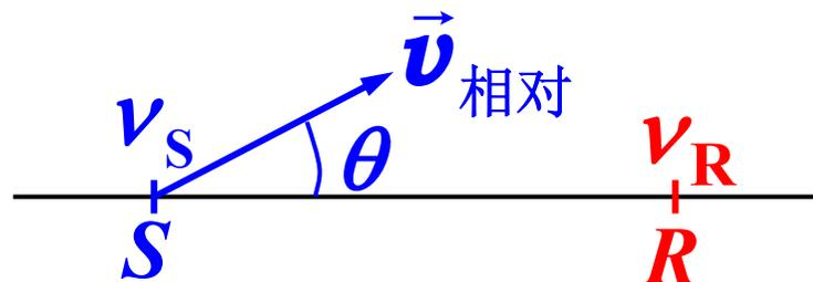
$$v_R = \frac{\sqrt{c^2 - v_{\text{相对}}^2}}{c - |\mathbf{v}_{\text{相对}}| \cdot \cos \theta} v_S$$
