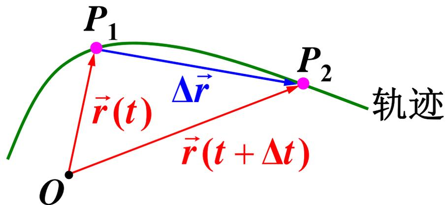
$$\Delta\vec{r} = \vec{r}(t + \Delta t) - \vec{r}(t) \left\{ \begin{array}{l} \text{大小 } |\Delta\vec{r}| = \overline{P_1P_2} \\ \text{方向 } P_1 \rightarrow P_2 \end{array} \right.$$
