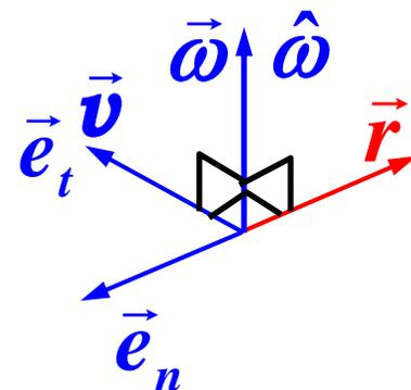
$$= R \omega (\vec{e}_n \times \hat{\omega}) = (R \vec{e}_n) \times (\omega \hat{\omega}) = \vec{\omega} \times \vec{r}$$
