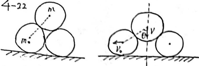
由动能定理:  $mg\Delta h = \frac{1}{2}mv^2 + 2 \times \frac{1}{2}m_0v_0^2$
